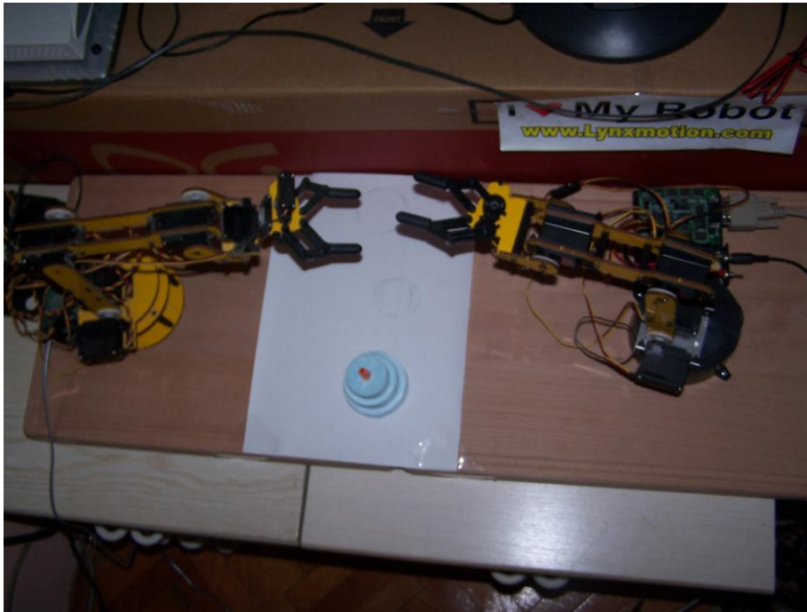
Figure 8.4. Two robotic arms used in the BCI experiments
