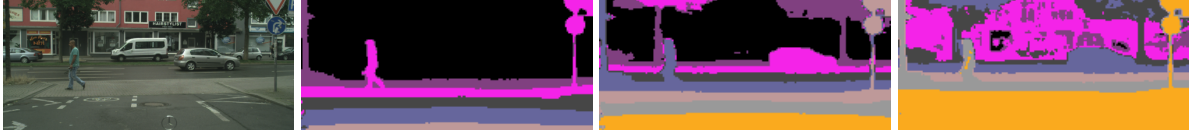
Figure 3.2: Visualization of the scale selection switches. From left to right: original image, switches for the three reference metric scales of 1m, 4m and 7m.
