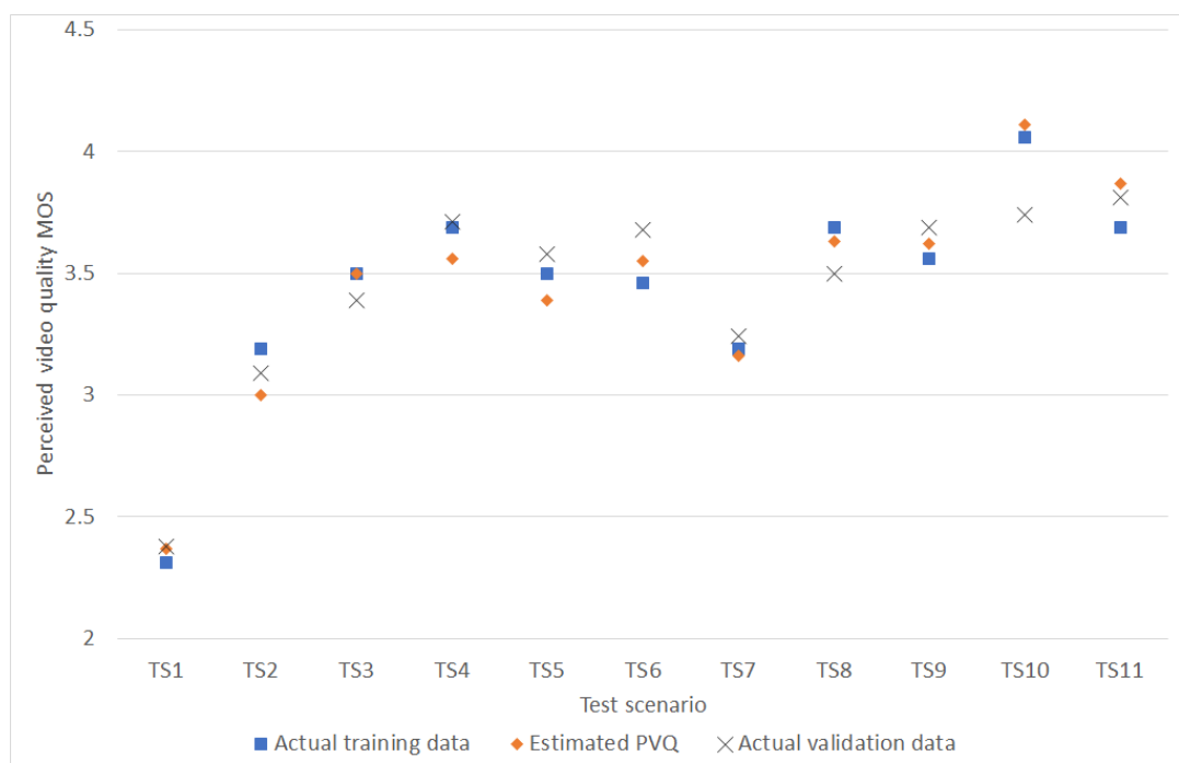
Figure 5.31: Comparison of actual and estimated perceived video quality mean ratings per test condition.
