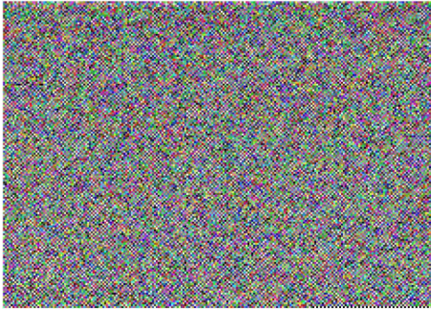
Figure 3. Squares in all simplified colors arranged in the pattern that was printed on a single big paper, illuminated by 707 different illuminations, and photographed.
