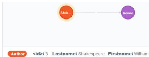
Fig.4. Result of creating a relationship between two nodes in Neo4j database
