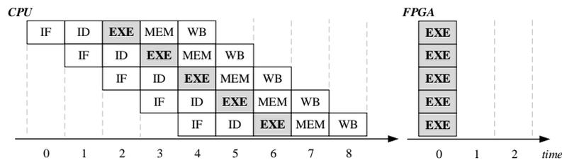
**Figure 2.7:** Instruction execution, CPU vs FPGA (from [122])
