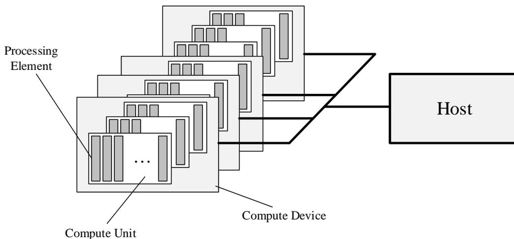
**Figure 2.3:** OpenCL platform model
