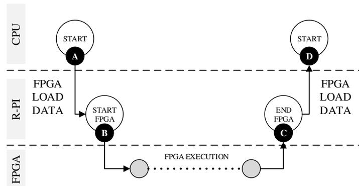
Figure 4.5: Time measurement points for the FPGA
