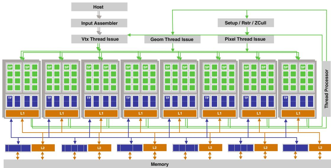
**Figure 2.2:** GPU Architecture of nVidia GeForce 8800 (from [90]). SP is a streaming processor, TF is a texture filtering unit, TA is a texture address unit.
