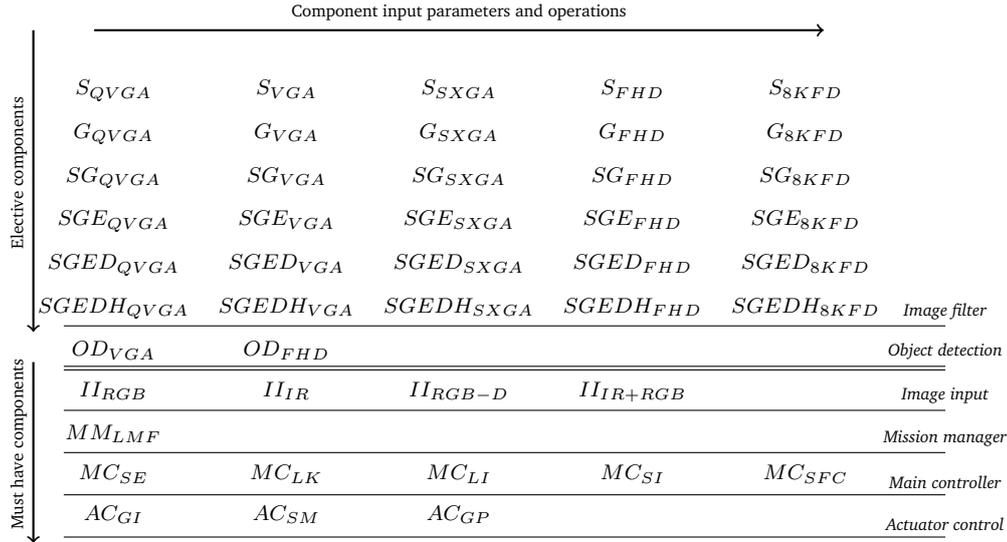
**Figure 5.1:** The Image filtering and the Object detection components let software architect make a lot of design choices, therefore these are named *elective components*, while the rest of components are obligatory and offer less design choices, these are named *must-have components*.
