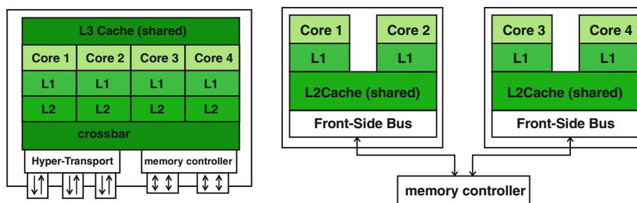
**Figure 2.1:** CPU Architecture, left image shows a hierarchical design multicore processor where cores share L3, and have their own L1 and L2 (AMD), while the right figure shows a design where two cores share L2, and communicate via a memory controller (Intel) (from [90]).
