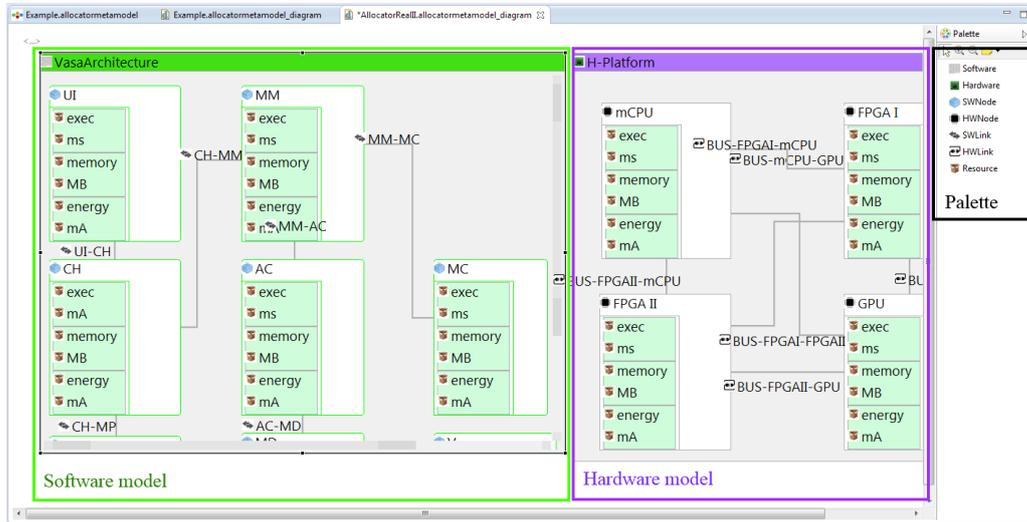
**Figure 5.3:** SCALL screen shot, showing software (left) and hardware (right) architecture side-by-side
