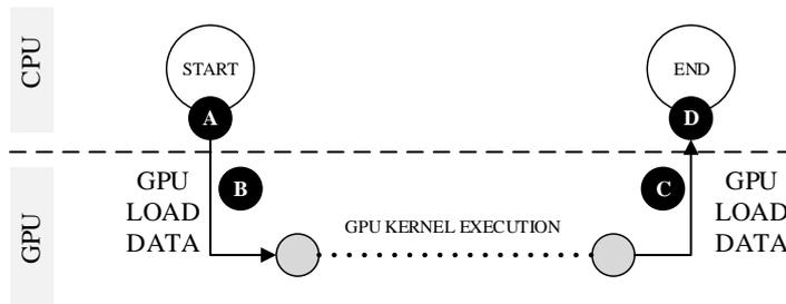
Figure 4.4: Time measurement points for the GPU
