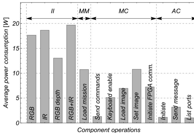
**Figure 4.12:** Remaining software components, average power consumption by a computing unit in Watts – barchart
