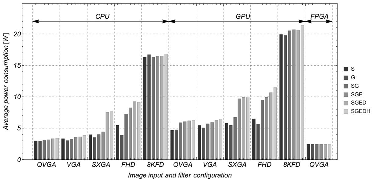
**Figure 4.10:** Image filtering component, average power consumption in Watts, for different inputs and operations – barchart
