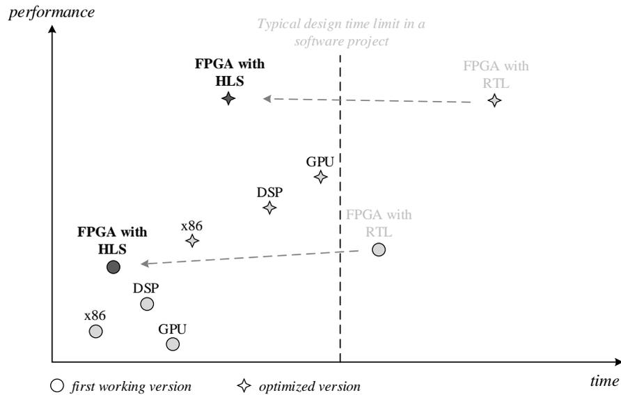
**Figure 2.5:** Design time vs. application performance (from [122]). A design shift from register-transfer level (RTL) model to hardware-level synthesis (HLS) dramatically reduced the design time while keeping the application performance.
