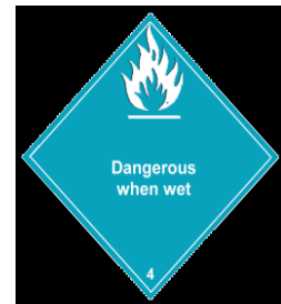
RFW-Dangerous when wet
