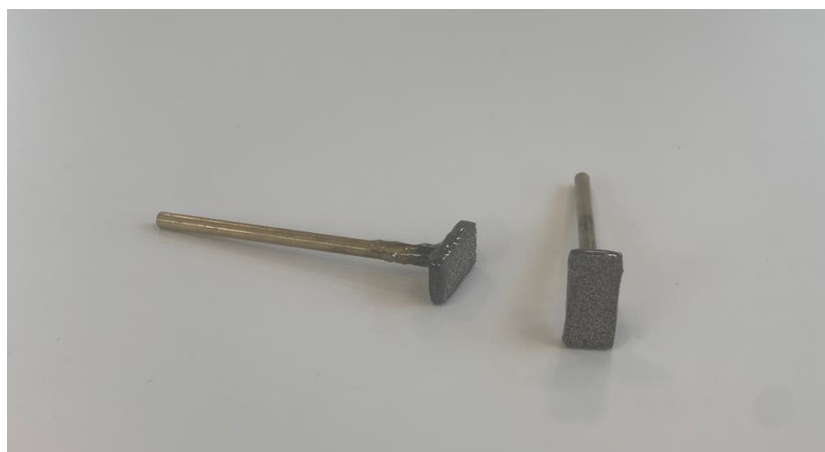
Figure 5. Ni foam electrodes
