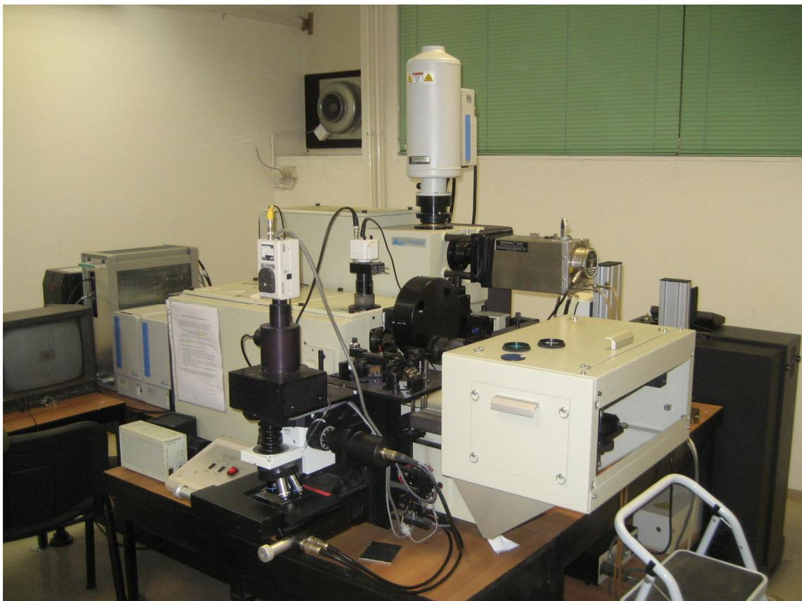
Slika 8. *Horiba JobinYvon T64000* mikro Raman sustav<sup>33</sup>
