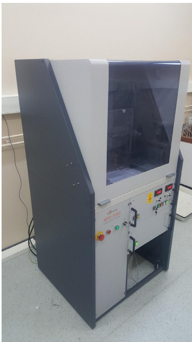
Slika 7. Difraktometar *ITALSTRUCTURES APD 2000*
