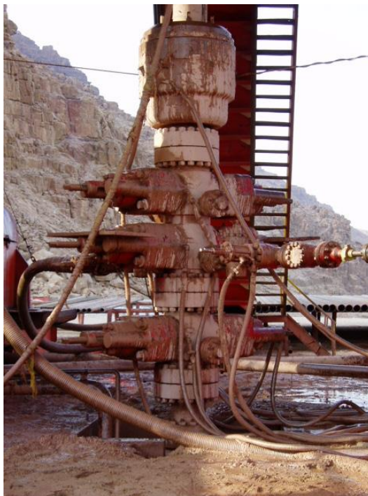
Slika 7-1. Preventerski sklop ( http://www.iwcfdrillengineer.com )
