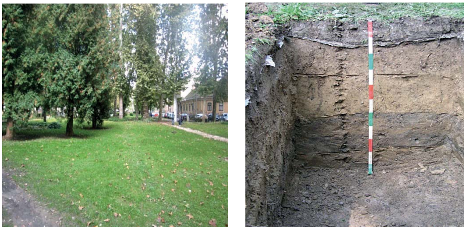
Slika 4. Krajolik i pedološki profil tla parka Lokacija: Sisak, dubina nanesenih slojeva je 90 cm Figure 4 Landscape and pedological profile of the soil of the park Location: Sisak, depth of the applied layers is 90 cm
