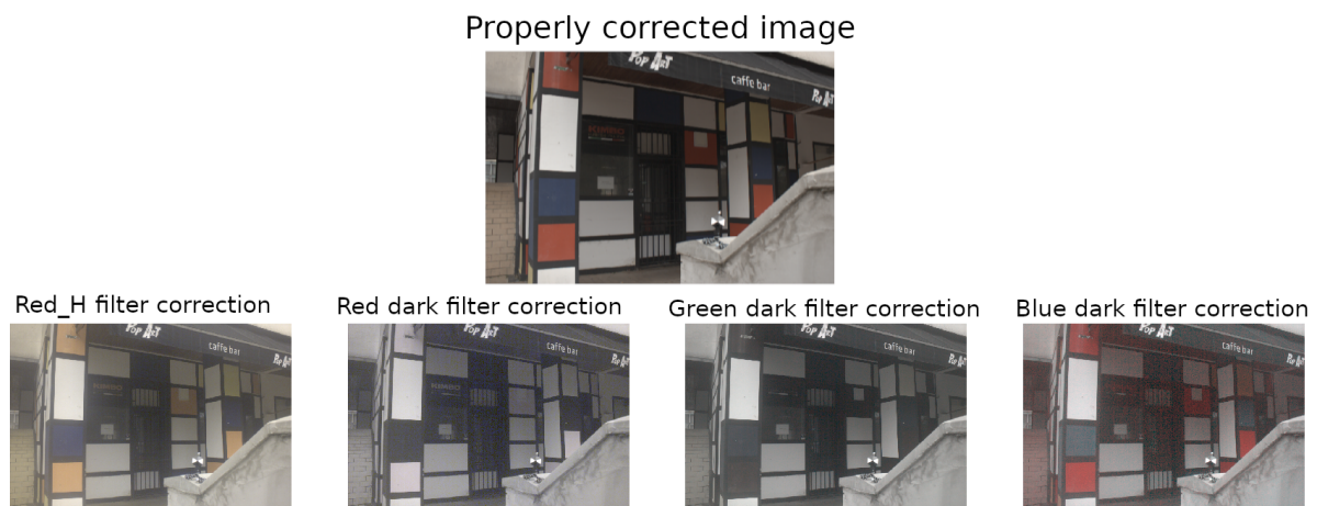
Figure 5.17: A couple of examples where the image cannot be properly corrected because of the extreme filters. The top row shows how the image should look and the bottom row the four situations where the image cannot be properly corrected.
