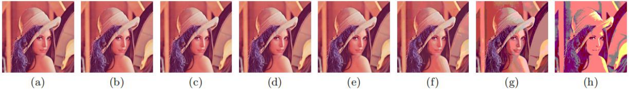
Figure 5. Influence of color reduction: (a) Without color reduction; (b) to (h) with color reduction, starting with only one bit in the red, green, and blue channel put to zero for (b) up to seven bits for (h).
