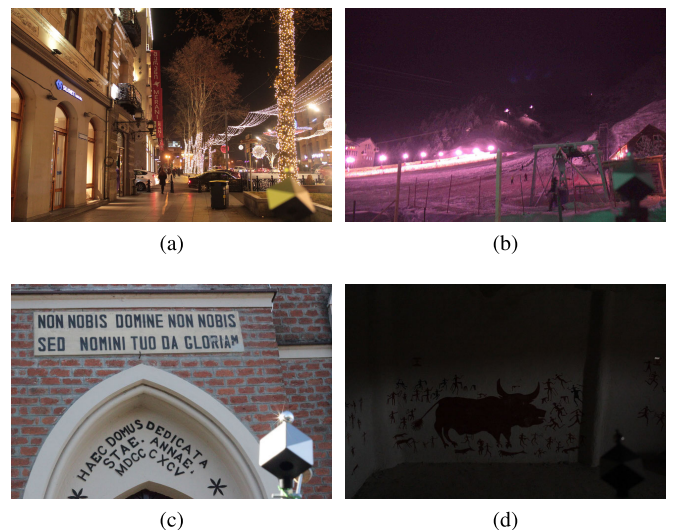
FIGURE 7. Examples of images that should be excluded from the dataset: a) the color target is illuminated by the local lantern from the near shop, the color is different from the lighting of the most of scene; b) the color target is illuminated by sources that have almost no effect on the lighting of the observed scene; c) overexposed color target; d) the overly dark image.
