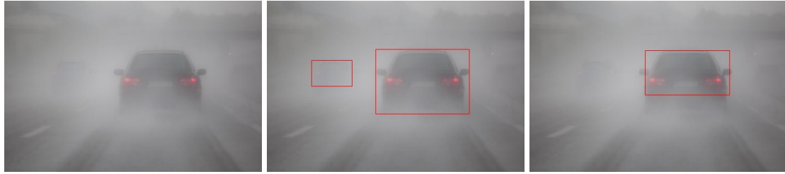
Figure 3.2: An example of an image from the RTTS section of RESIDE dataset. On the left is the image, in the middle is the image with ground truth bounding boxes shown for all objects, and right is the detections made in the hazy image.
