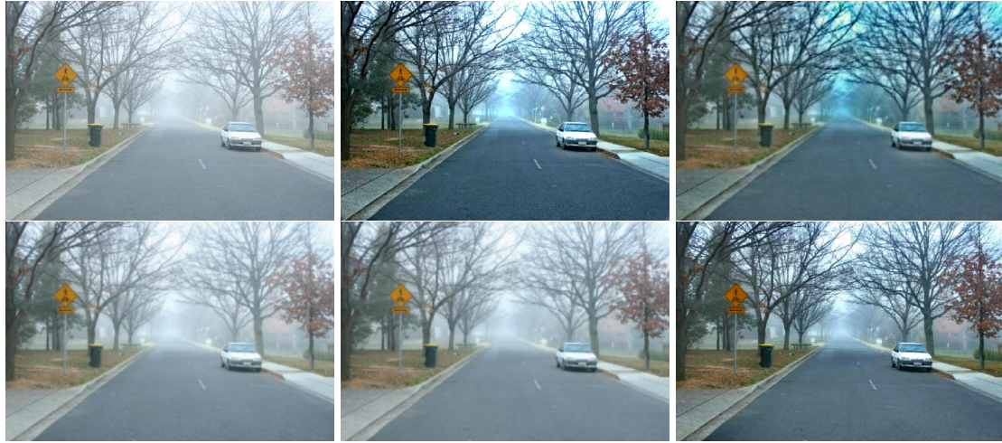
Figure 6.6: Top left is the original image, top middle image dehazed using VarDCP, and top right using Unsupervised DCP. Bottom left is dehazed using FFANet, bottom middle using Dehazeformer, and bottom right using MSCNN. Note that the biggest improvements seem to be from the VarDCP method and the unsupervised DCP method, while the smallest improvements seem to come from the FFANet and Dehazeformer.
