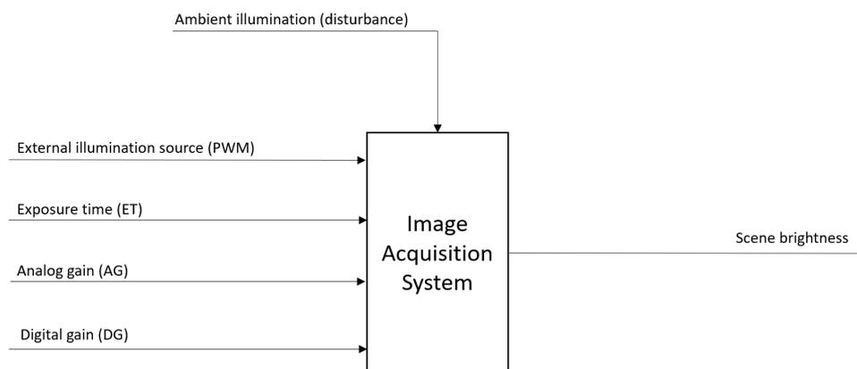
**Figure 2.4:** Block schematics of the image acquisition system
