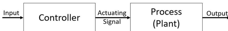
**Figure 2.5:** Block schematic of an open-loop control system
