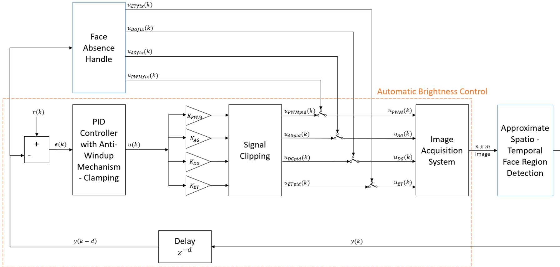
**Figure 5.3:** The complete automatic brightness control block scheme, with the split-range PID controller, anti-windup and clipping mechanism in orange, and face region detection and the face absence handle in blue
