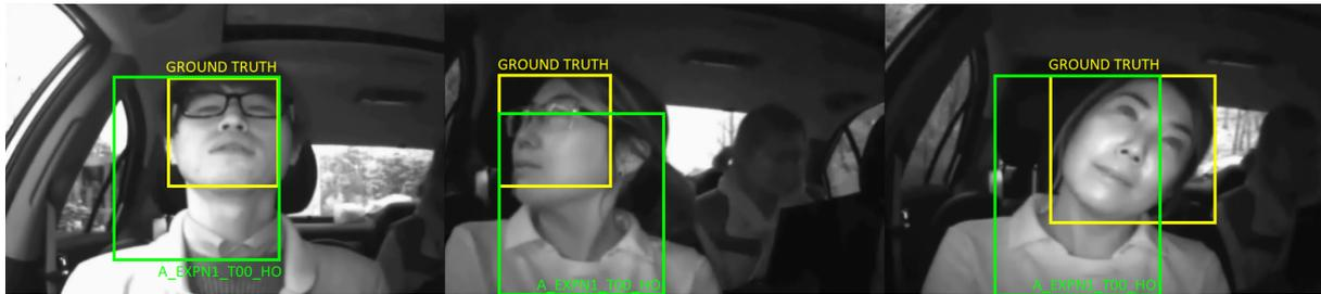
**Figure 4.10:** Unsuccessful detection example with ground truth face region bounding box (yellow) and proposed variant *A\_Expn1\_T00\_H0* face region bounding box (green), with the Viola-Jones not detecting faces
