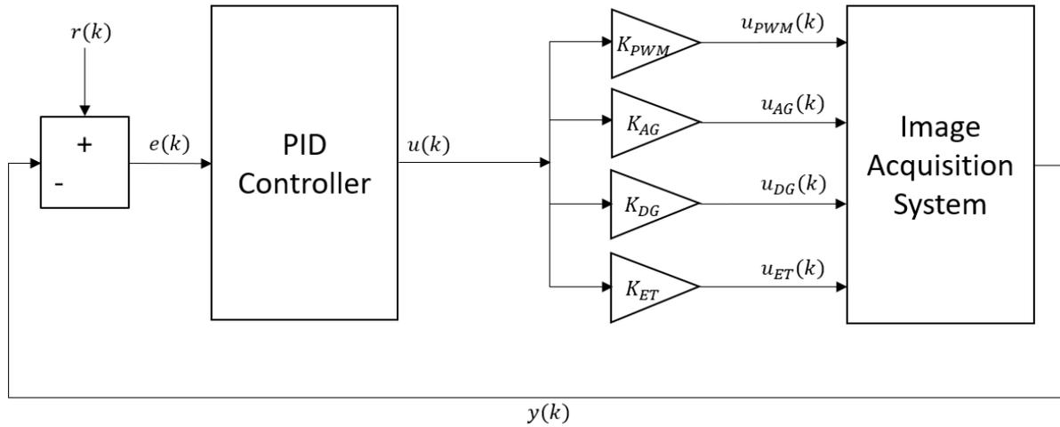
**Figure 5.1:** Simple split-range PID controller block scheme
