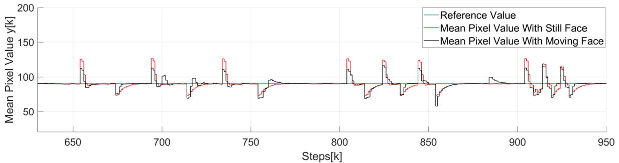
**Figure 5.8:** Enlarged brightness response change caused by a controllable disturbance with control and region detection with a still and moving face
