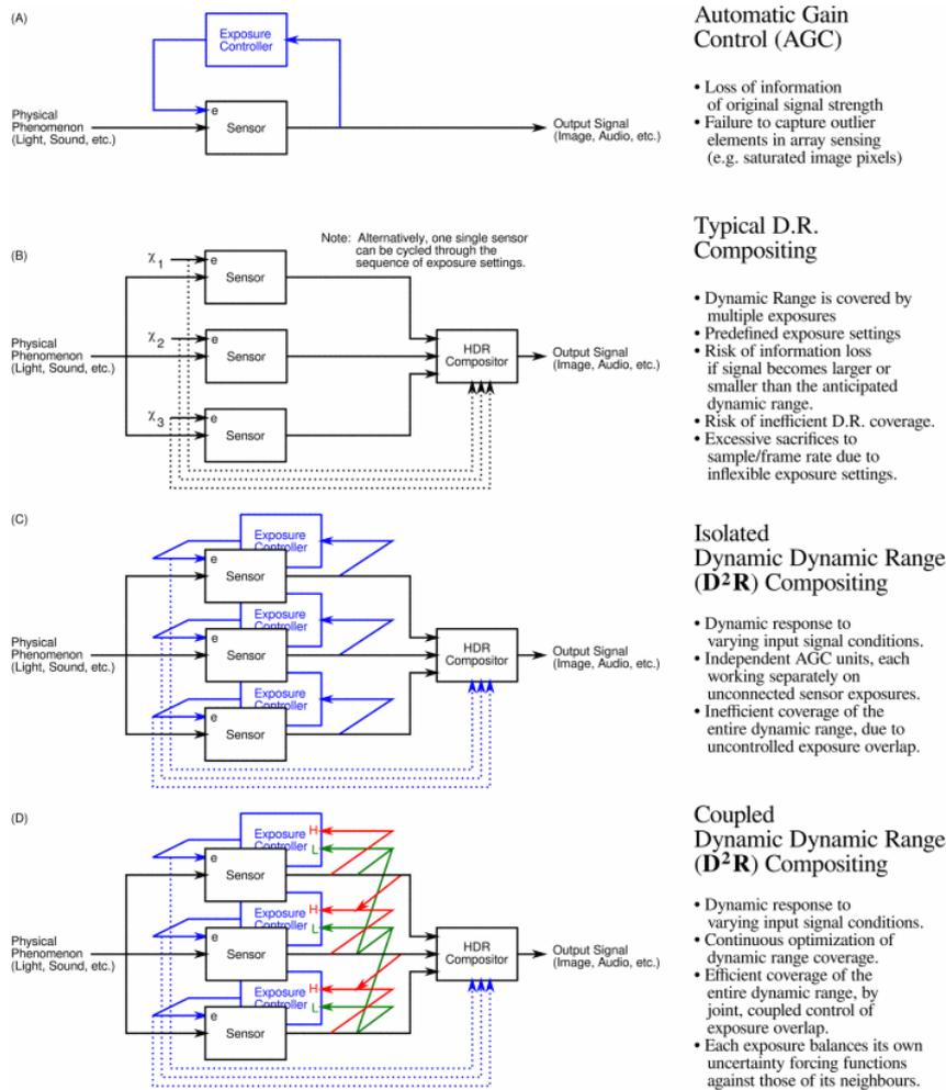
**Figure 3.4:** Schematic of Janzen’s algorithm for multiple exposure feedback system that describes automatic gain control (A), HDR compositing (B), multiple feedback exposure time loops (C), and the coupling of the multiple feedback exposure time loops (D) [55]
