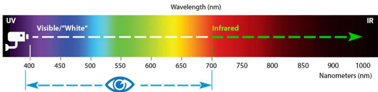
Figure 2.2: Visible wavelengths for a human eye and a camera [21]
