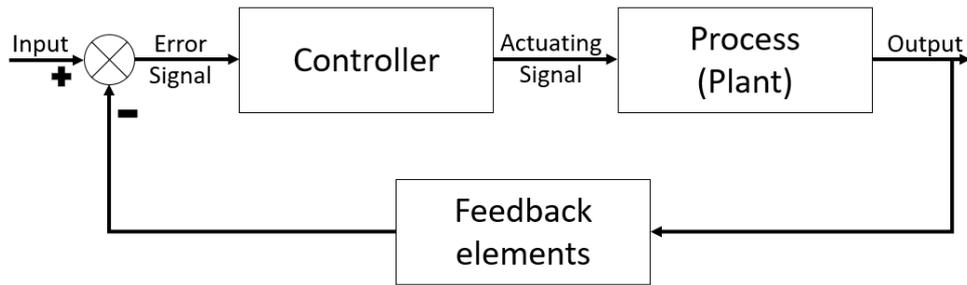
**Figure 2.6:** Block schematic of a closed-loop control system
