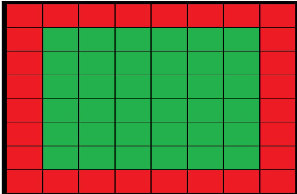
**Figure 5.6:** Fixed region of interest (green) in a scene used for setups with face region detection disabled, where outer tiles (red) are not included in the calculation
