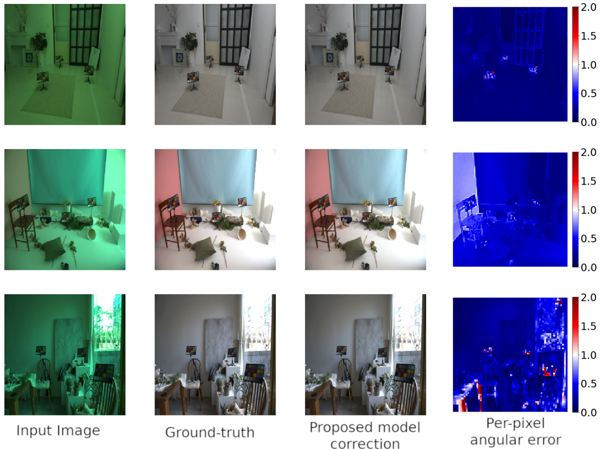
Figure 6.13: Visual comparison of Image-approach model-corrected image and ground-truth corrected image on the LSMI dataset. The angular error heatmap for each image is also shown. The max angular error in the heatmaps is 2^\circ . All images have been tone-mapped for better visualization.
