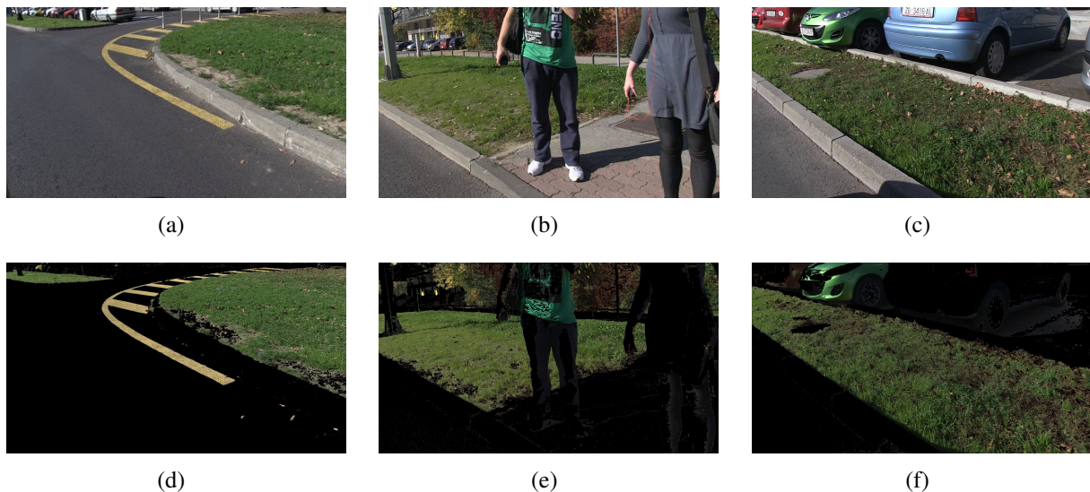
Figure 3.11: Examples of vegetation detection using only green vegetation for training.
