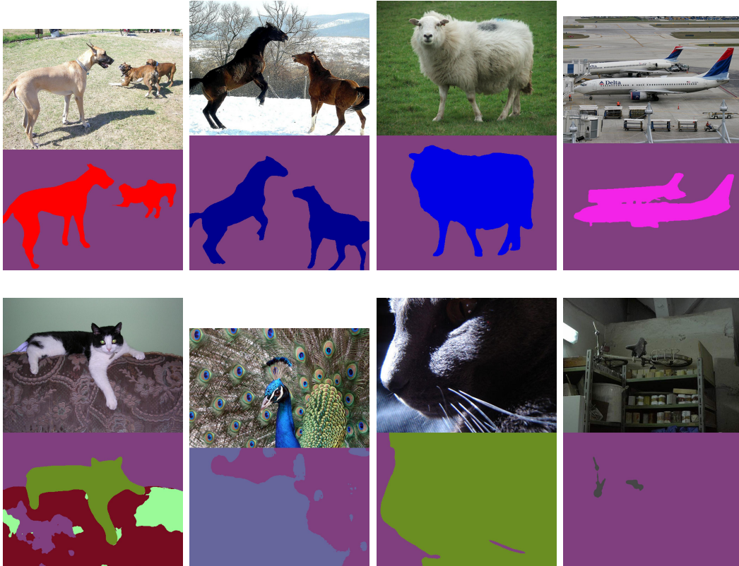
Figure 4.12: Example predictions on the Pascal VOC 2012 test set. Top row shows instances of easy examples for dog, horse, sheep and airplane classes. Bottom row shows instances of hard examples for sofa, bird, cat and bicycle classes. Note that most errors are caused by insufficient information on cropped objects, large object scale and pose variance and rare context around the object.
