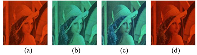
Figure 7. Examples of data augmentation by illumination simulation on images generated by the proposed dataset generator: (a) the linear raw image of the printed photography taken under the red light, (b) the simulation of taking the image under the white light by applying Eq. (5) to the previous image, (c) the linear raw image of the printed photography taken under the white light, and (d) the
