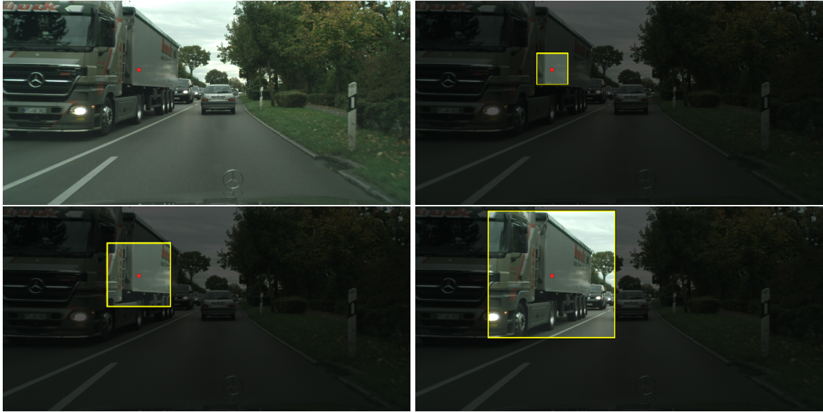
Figure 1.2: Top left: a typical input image presented at the model input. Classification of the pixel marked in red is considered for a model with receptive field 200 \times 200 pixels. The receptive field is visualized in the original (top right), two (bottom left) and four (bottom right) times subsampled images.
