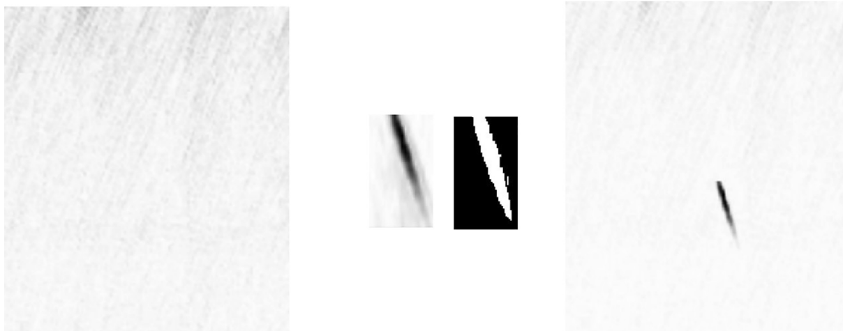
Fig. 2. Example of (from left to right) an empty canvas (B-scan without defects), an extracted defect and its binary pseudo mask, and resulting generated image.
