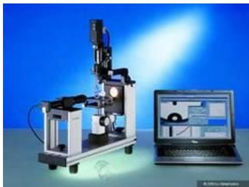
Slika 3.2.4. OCAH 200 Data Physics Contact Angle System
