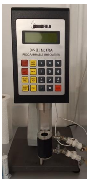
Slika 11. Reometar DV-III Ultra Rheometer by AMETEK Brookfield
