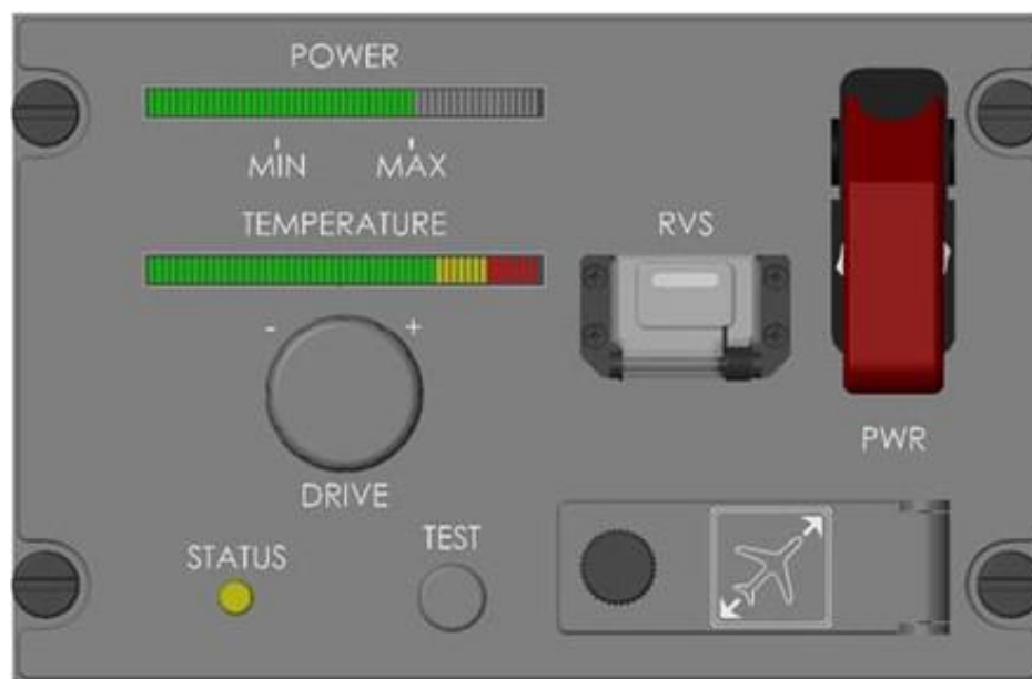
Figure 7. Publicly available WheelTug cockpit panel design 79
