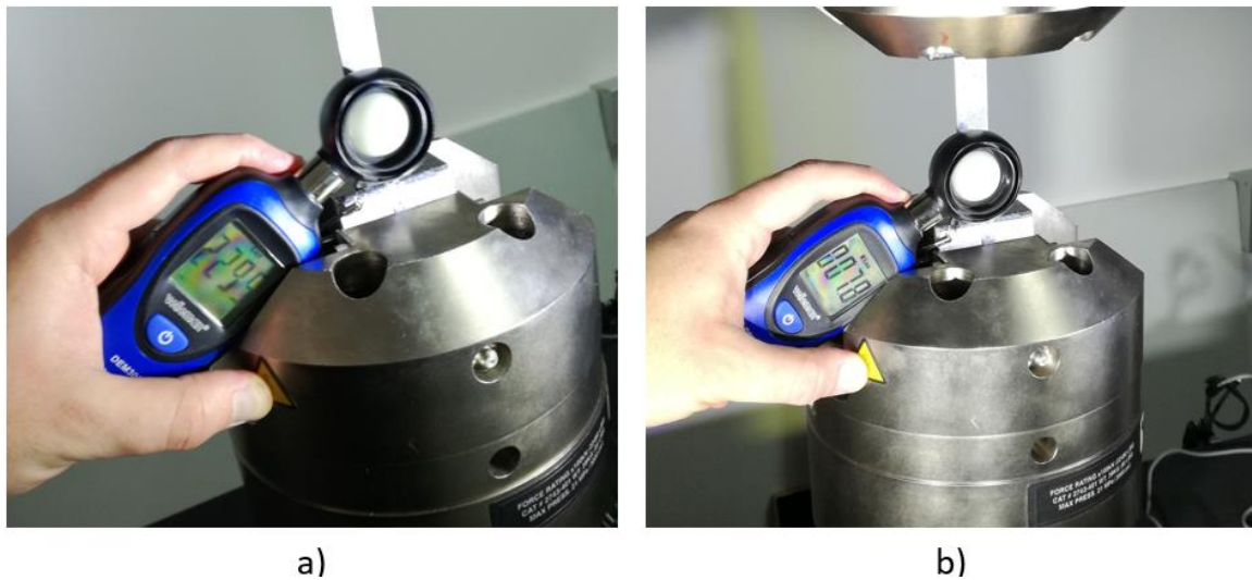
Figure 14. Illuminance with a) Aramis 4M integrated light b) additional 2 x 50W led light
