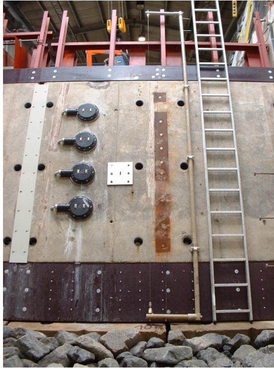
Figure 2.11: Photograph of the vertical wall from the breaking wave impact experiment [6] (PAPER 6), with holes going through the wall that are not included in the present CFD study.
