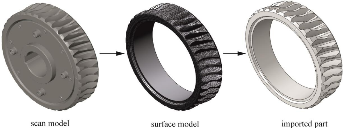
Figure 65. Worm wheel model creation [1]
