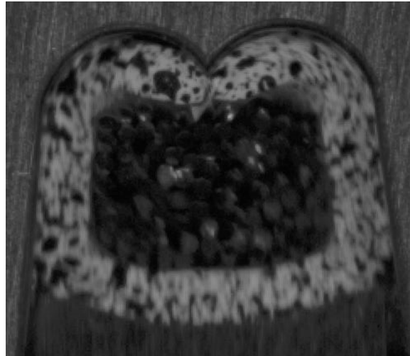
Figure 38. Blurred image captured by camera at crimping speed of 50 mm/s
