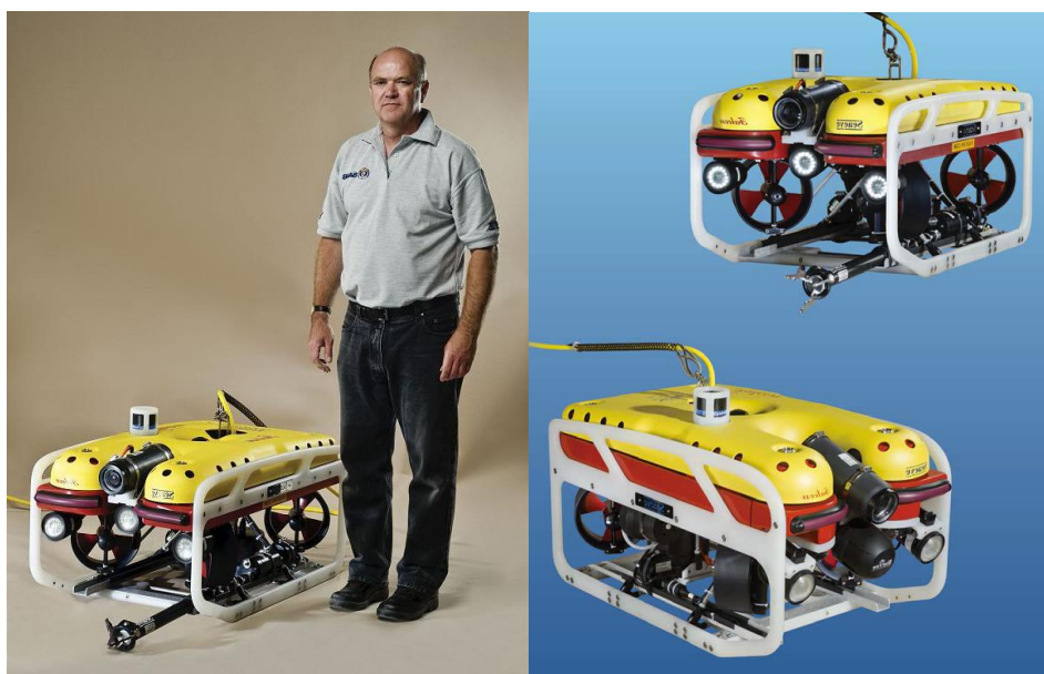
Slika 2.8 SAAB Seaeye Falcon Observation class ROV (100kg)
