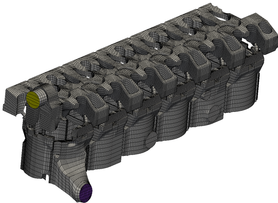
Figure A4: Engine cooling: finite volume mesh, inlet surface is purple, outlet is yellow.
