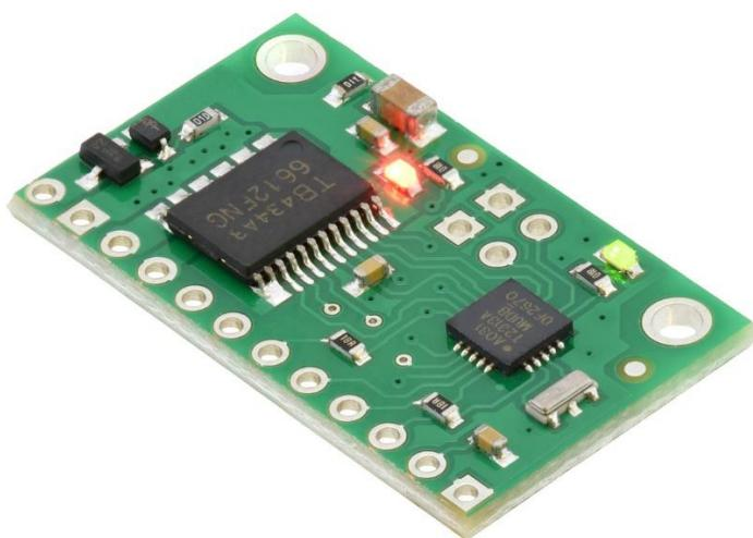
**Slika 40. Pololu Qik 2s9v1 Dual Serial Motor Controller[19]**
