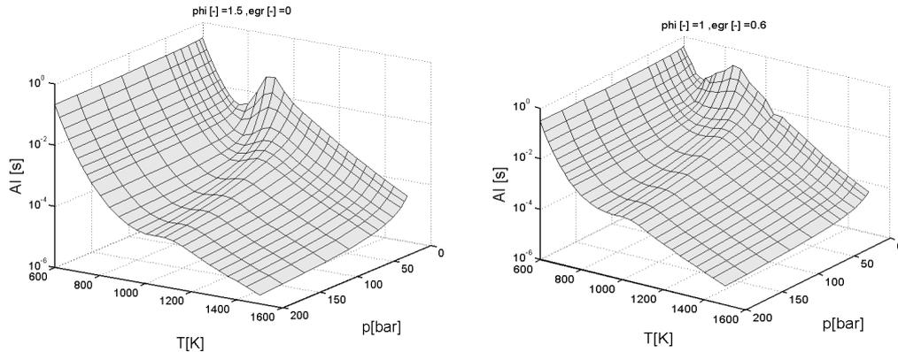
Figure 3-2 n-heptane table for  $\phi = 1.5$ , and  $EGR = 0$  (left) and  $EGR = 0.6$  right using Curran et al. mechanism
