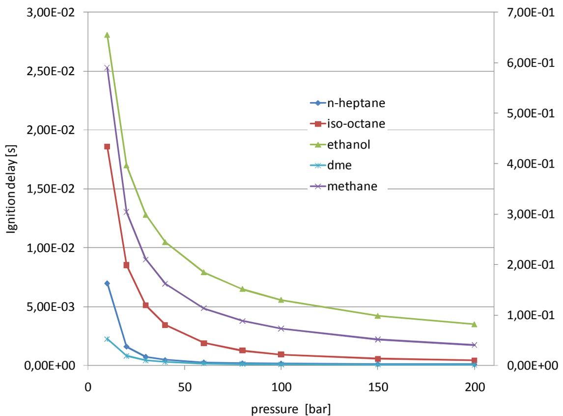
Figure 2-3 Pressure dependence of autoignition of selected fuels
