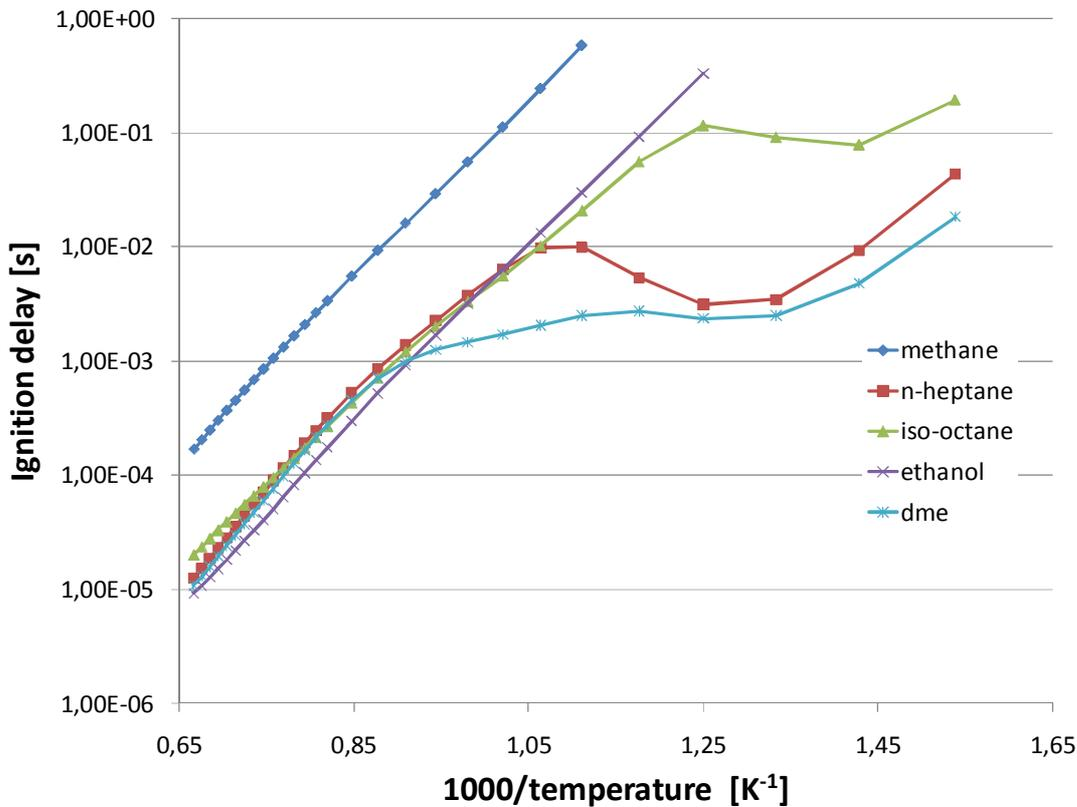
Figure 2-2 Temperature dependence of autoignition of selected fuels
