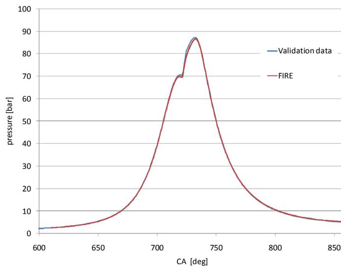
Figure 3-14 Validation data and calculated pressure profile
