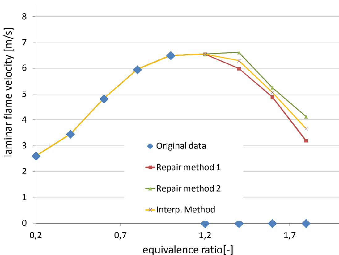
Figure 2-17 Sample set of results with missing more data (also ethanol but the case with equivalence ratio)
