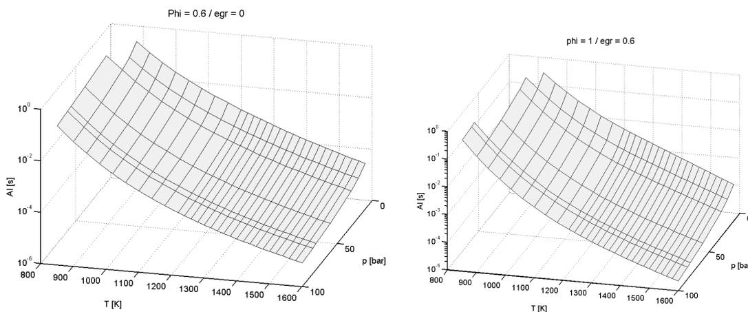
Figure 3-6 Methane autoignition tables with variable pressure and temperature and with phi = 0.6 and egr = 0 (left), and with phi = 1 and egr = 0.6 (right)
