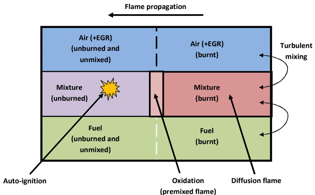
Figure 2-20 ECFM-3Z model description of mixing zones [32]
