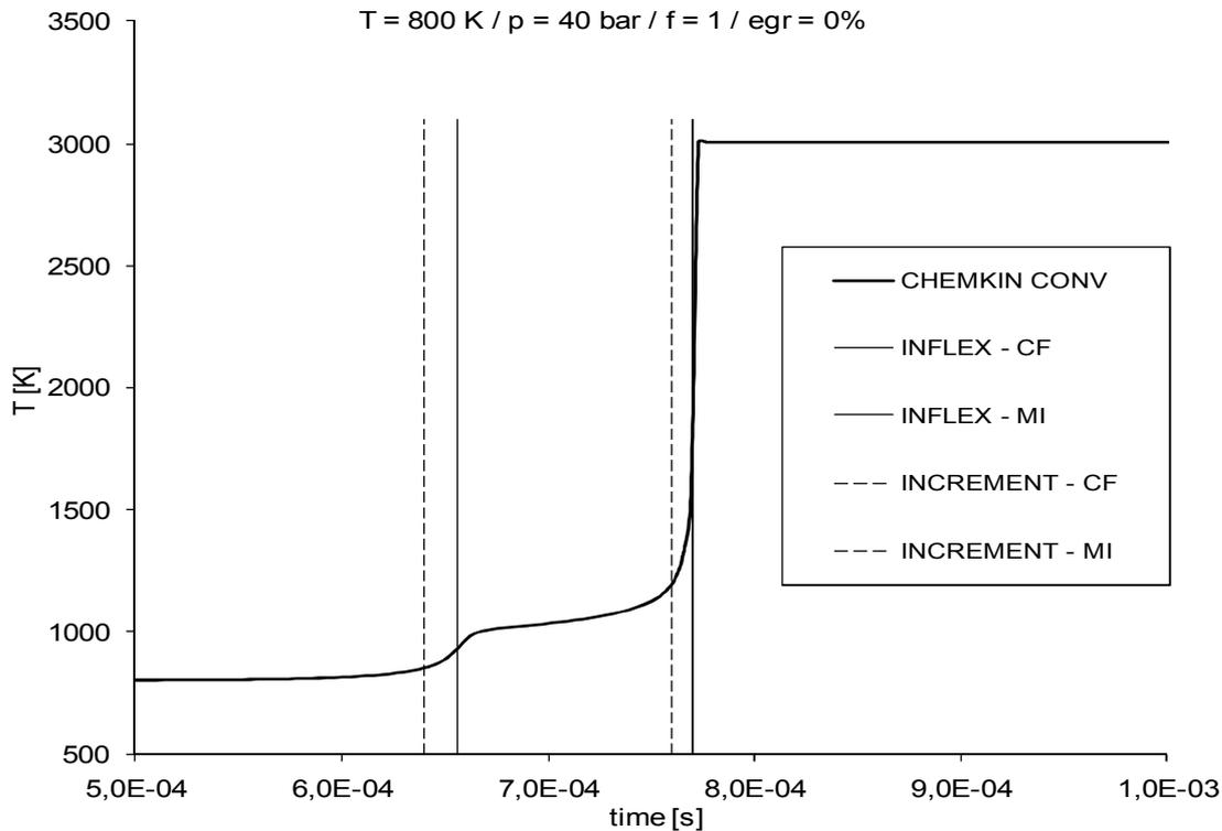
Figure 2-1 Ignition tracking criteria compared
