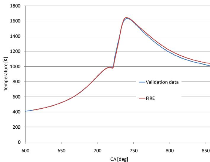
Figure 3-13 Validation data and calculated temperature profile
