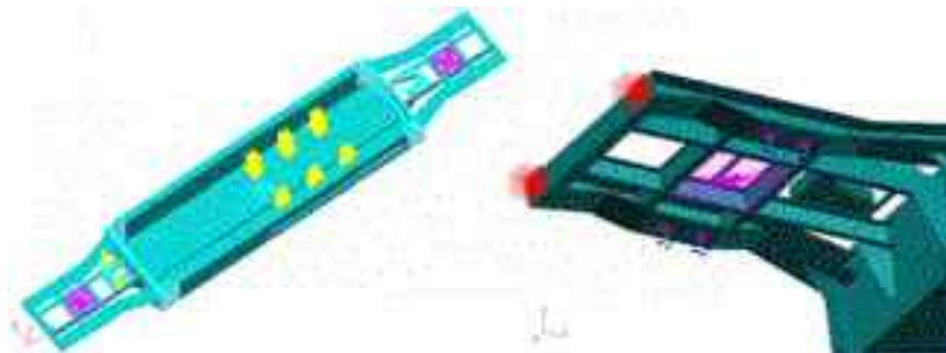
Figure 5 Wagon FE model – general view and model of boundary conditions (constraints and loads).
