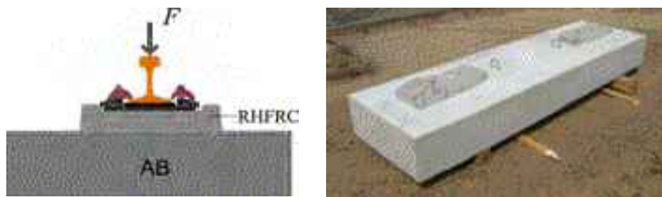
Figure 7 A track prototype on a concrete surface – ECOTRACK [2]
