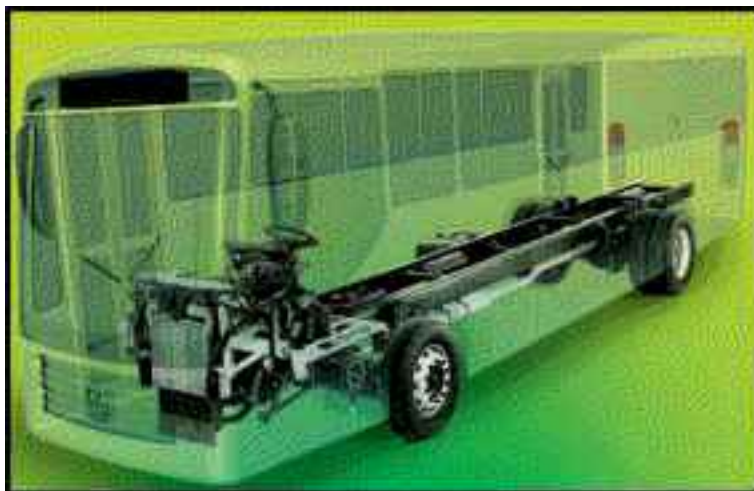
Figure 1 Typical front engine bus configuration [1]
