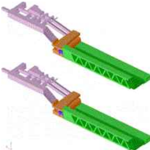
Figure 7 FE model of the part of the wagon after constructional modifications – top and bottom views.
