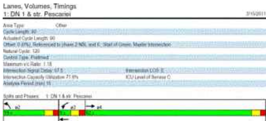
Figure 3 Example of traffic light simulation in Synchro
