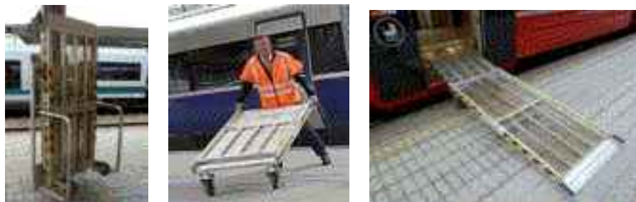
Figure 1 Platform based Ramp NSB, Norway
