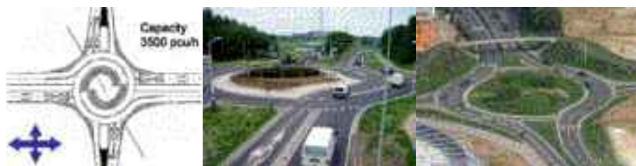
Figure 2 Basic concept of turbo roundabout and its design in the Netherlands and Germany
