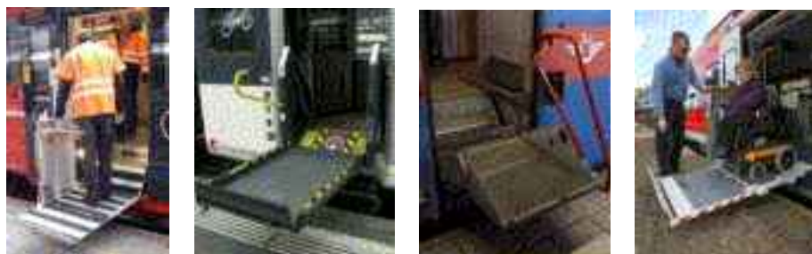
Figure 4 Examples for vehicle based lifts in Norway, Switzerland, Sweden and Germany
