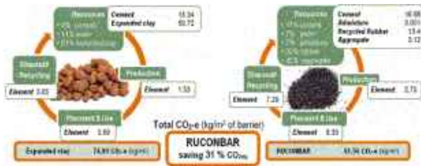
Figure 8 Comparison of noise barriers production process: expanded clay vs. recycled rubber
