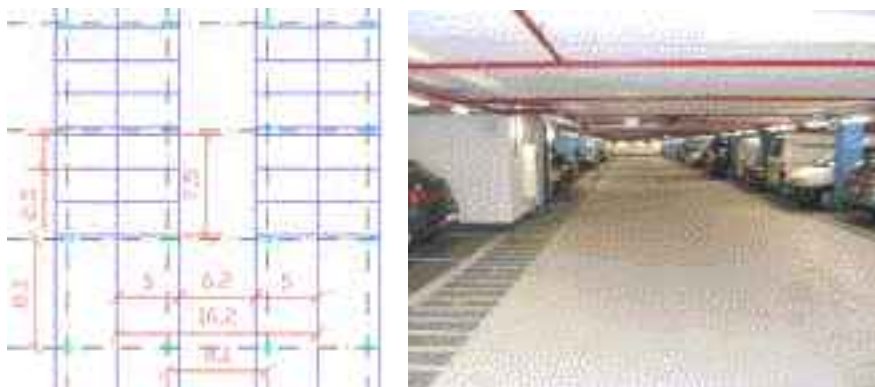
Figure 5 Example of a construction column grid for buildings with underground garage level(s). Realized: Opernturm garage, Frankfurt Main
