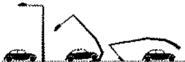
Figure 11 Low energy absorbing columns behaviour [6]
