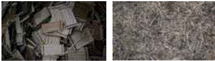
Figure 3 a) Industrial steel fibres (Dramix RC 65/35 BN); b) Recycled steel fibres (Gumiimpex GRP)
