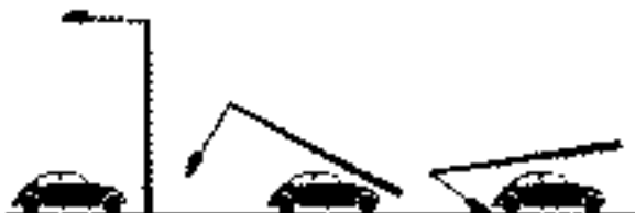
Figure 4 Non-energy absorbing column behaviour [6]
