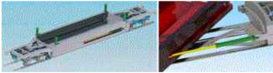
Figure 3 Geometrical model of the special railway wagon with a rotatable platform – view of four vertical pin joint type locks and a part of the wagon structure prepared for loading and unloading operations.
