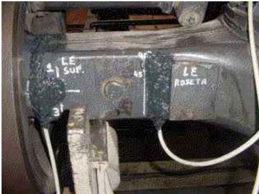
Figure 4 Detail of the instrumentation of the left hand side of the rear axle beam – same instrumentation was made on the right hand side of the component
