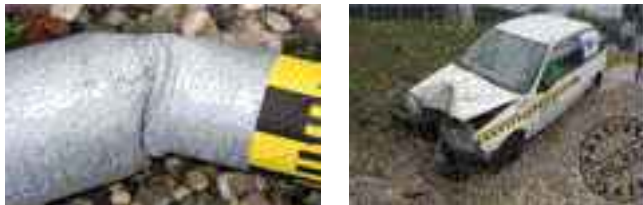
Figure 6 Column detail and vehicle after the crash test [7]
