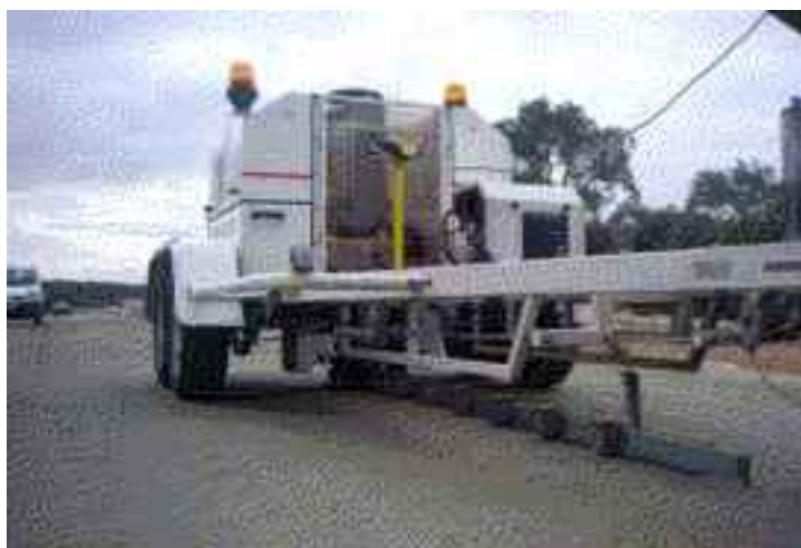
Figure 1 Falling Weight Deflectometer equipment.
