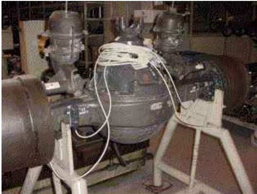
Figure 3 General view of the instrumented rear axle beam
