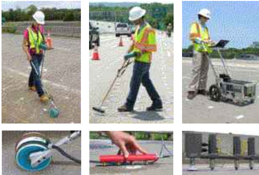
Figure 2 HCP testing and reference electrode (left), ER measurement and Wenner probe (middle), and USW measurement and PSPA (right).
