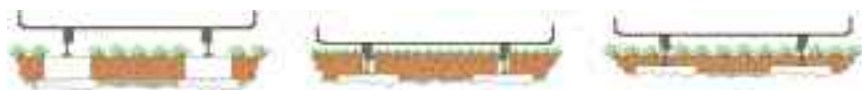
Figure 3 Schematic diagram of the limited space between the tram underbody and the vegetation layer, depending on the vertical spacing between top of rail and vegetation (From left to right: low vegetation, high vegetation and intermediate vegetation)
