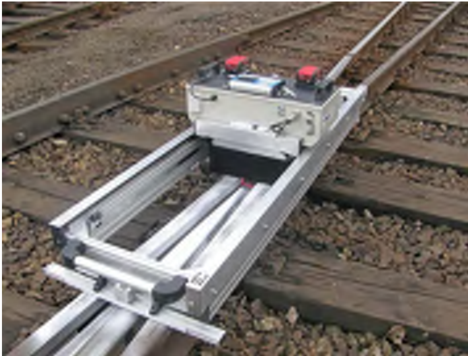
Figure 6 Optical system for track and turnout measurement
