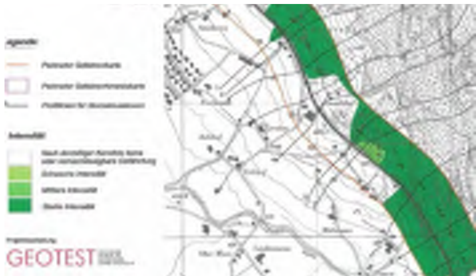
Figure 5 Intensity map of rockfall for 100 year return period shows at the area of projected nets a high intensity Middle shallow landslide intensity means slight break failure depth M between 0.5 < M < 2 m and flow height h up to 1 m. From the landslide working group suggestion AGN [11] impact pressures up to 60 \text{ kN/m}^2 have to be considered for middle intensity. The rockfall hazard map gives rockfall energies with high intensity which means energies larger than 300 \text{ kJ} (see Table 1). From rockfall field investigation and simulation results the design energy results in 2'000 \text{ kJ} for the net impact.
