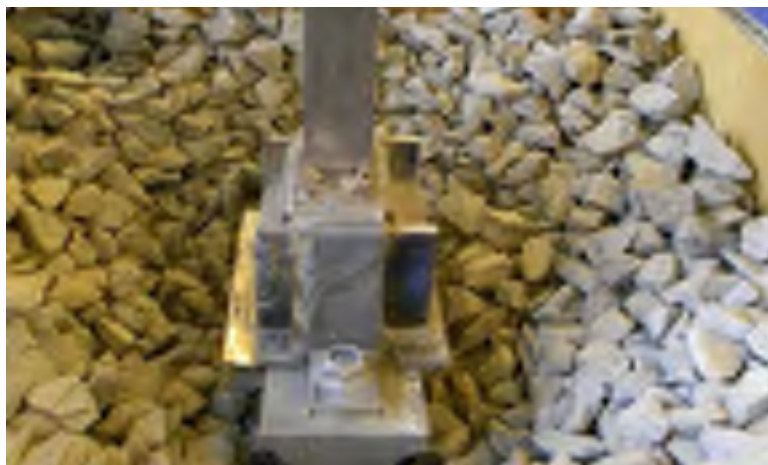
Figure 3 Test of tearing resistance in ballast
