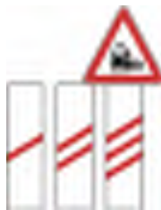
Figure 2 Approaching the level crossing without barriers or semi-b.
