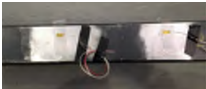
Figure 3 Primary suspension spring leaf instrumentation
