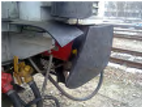
Figure 3 Fig.3. Crash buffer of a sleeping carriage operated in Bulgaria since April 2013
