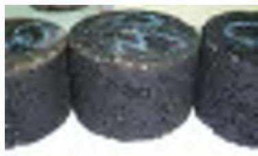
Figure 2 Laboratory asphalt specimens
