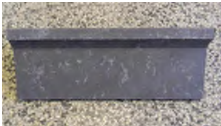
Figure 4 Plastic sleeper anchor after abrasion resistance test
