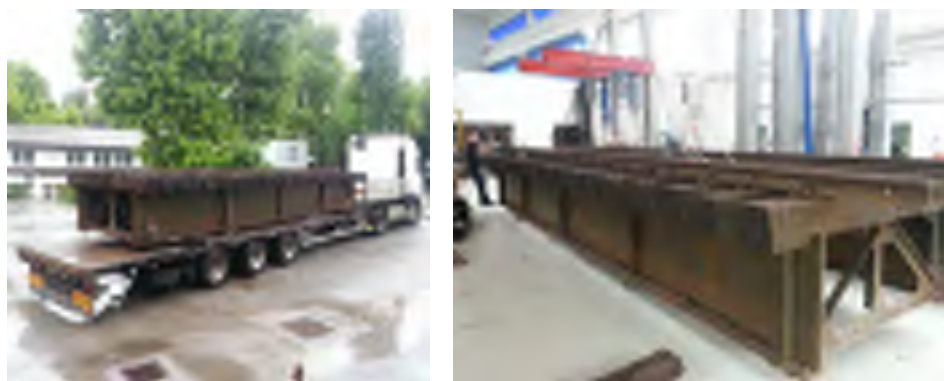
Figure 2 Bridge transported into laboratory
