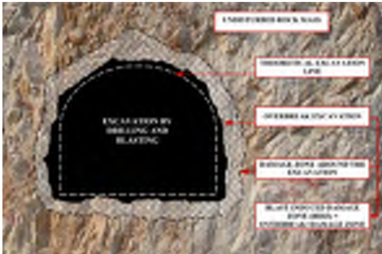
Figure 1 Schematic view of Blast-Induced Damage Zone (BIDZ)
