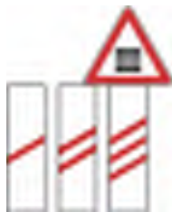
Figure 1 Approaching the level crossing with barriers or semi-barriers.
