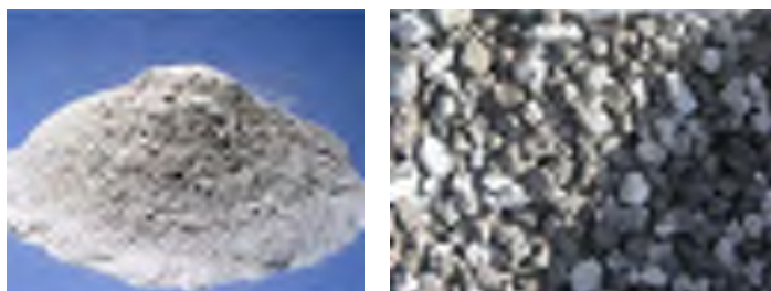
Figure 1 Industrial waste materials: fly ash (left) and slag (right)
