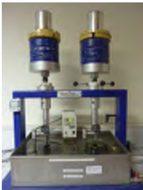
Figure 1 Machine to measure the indentation according to the standards EN 12697-20 and EN 12697-21
