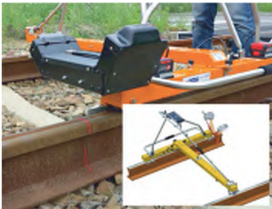
Figure 2 Track geometry and rail head profile trolley
