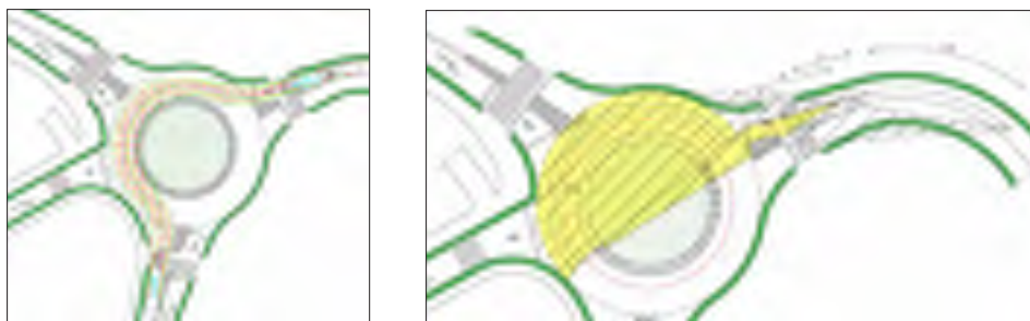
Figure 5 Turning paths for design vehicle (left) and visibility control (right) – examples for approach 1 [13]
