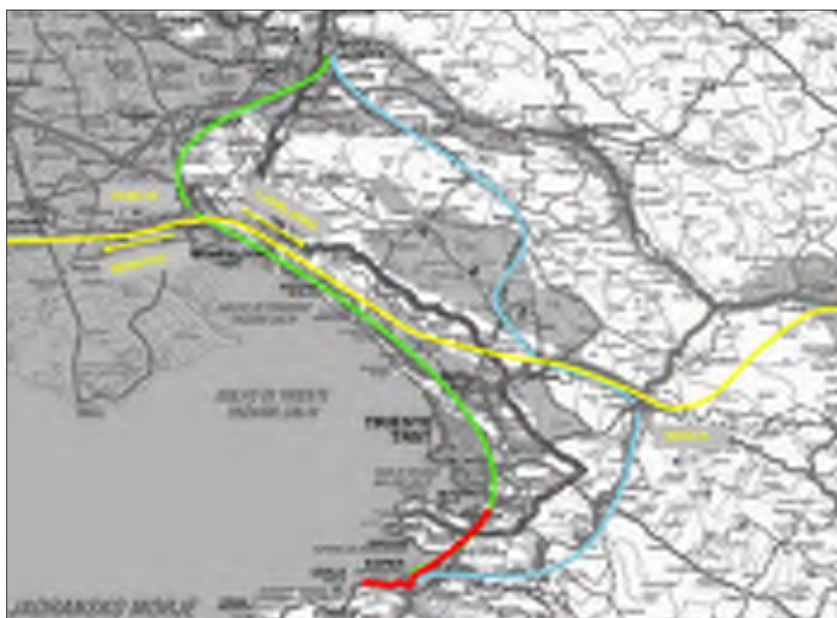
Figure 4 Trieste rail ring (blue and green), high speed rail (HSR) Venice-Ljubljana (yellow) and the missing connection between Trieste/Aquilinia and Koper (red).
