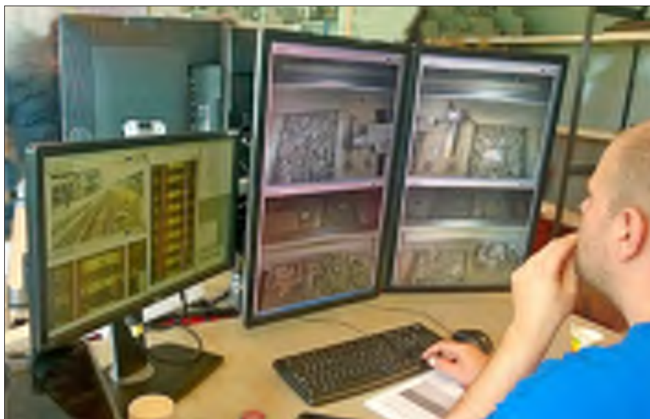
Figure 5 Video inspection results analysis – synchronised with track geometry measurement, and other data
