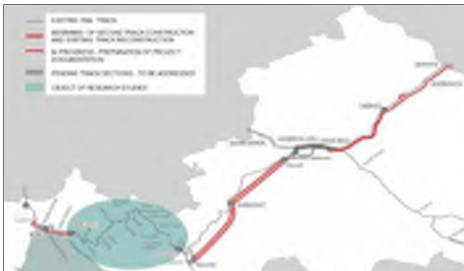
Figure 3 Activities on design of construction, reconstruction and modernization of the corridor RH2, State Border-Botovo-Zagreb-Rijeka [6]
