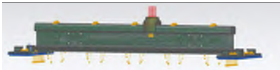
Figure 6 3D model of the force sensor ready for analysis with defined finite element meshes, loading and boundary conditions, and mating conditions
