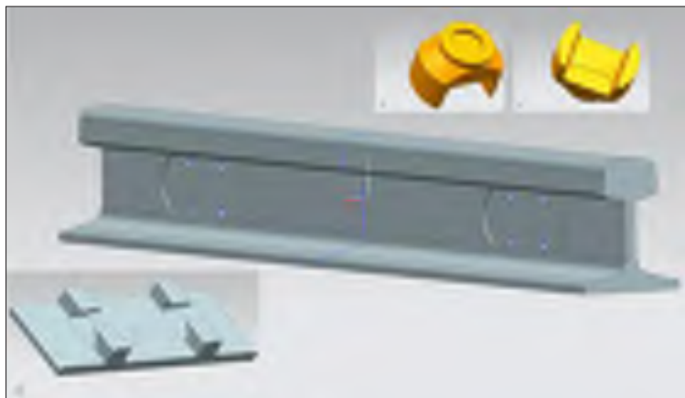
Figure 5 3D models of the force sensor assembly
