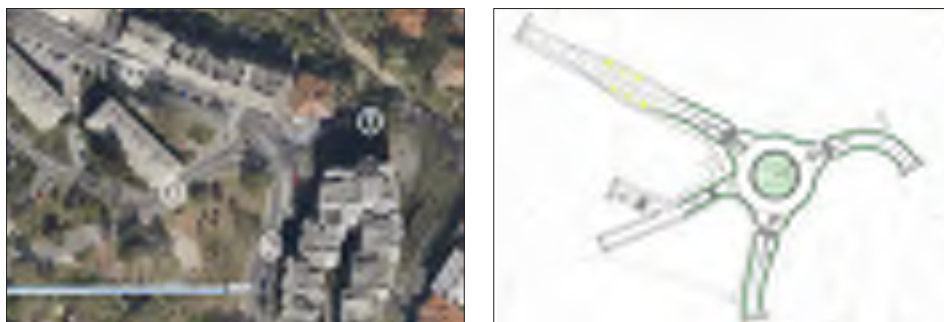
Figure 4 Present situation at intersection Case study 2 (left) and roundabout design at location (right) [13]
