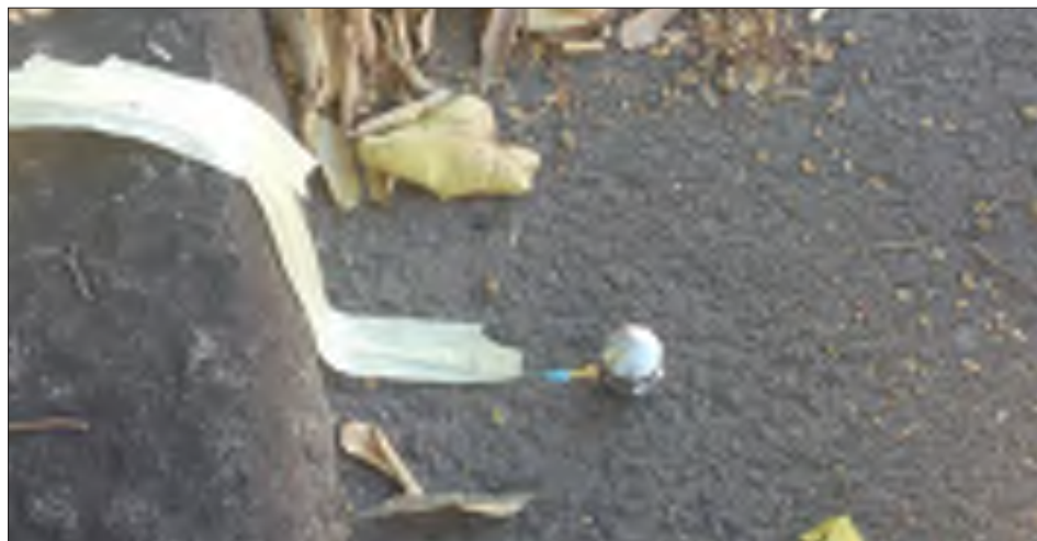
Figure 17 Placements of an accelerometer
