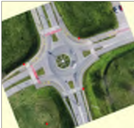
Figure 3 Aerial photo with marked control points taken by UAS
