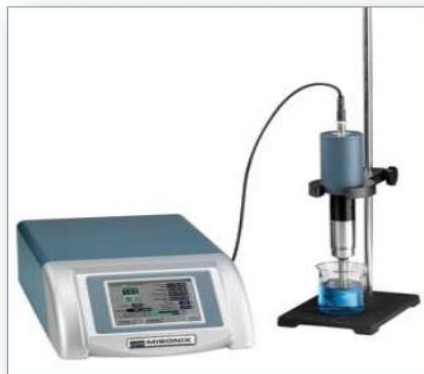
Slika 2. Ultrazvučni procesor model S-4000 (MisonixSonicators, Newtown, Connecticut, SAD)
