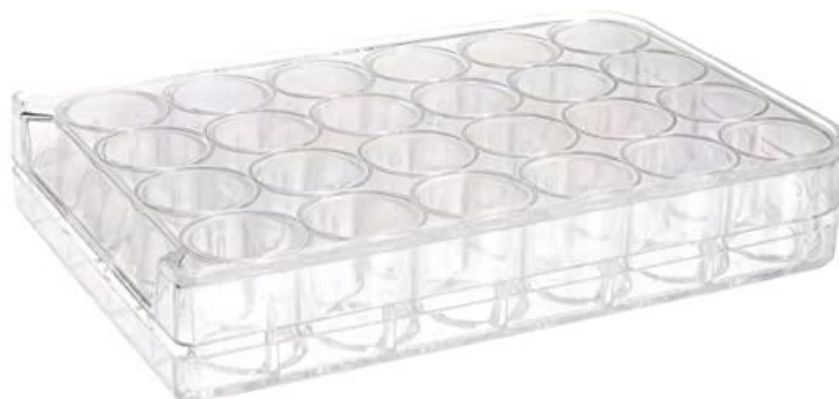
Slika 7. Prikaz ploče s 24 jažice ( 24-well plate ) (Anonymous 6, 2022)
