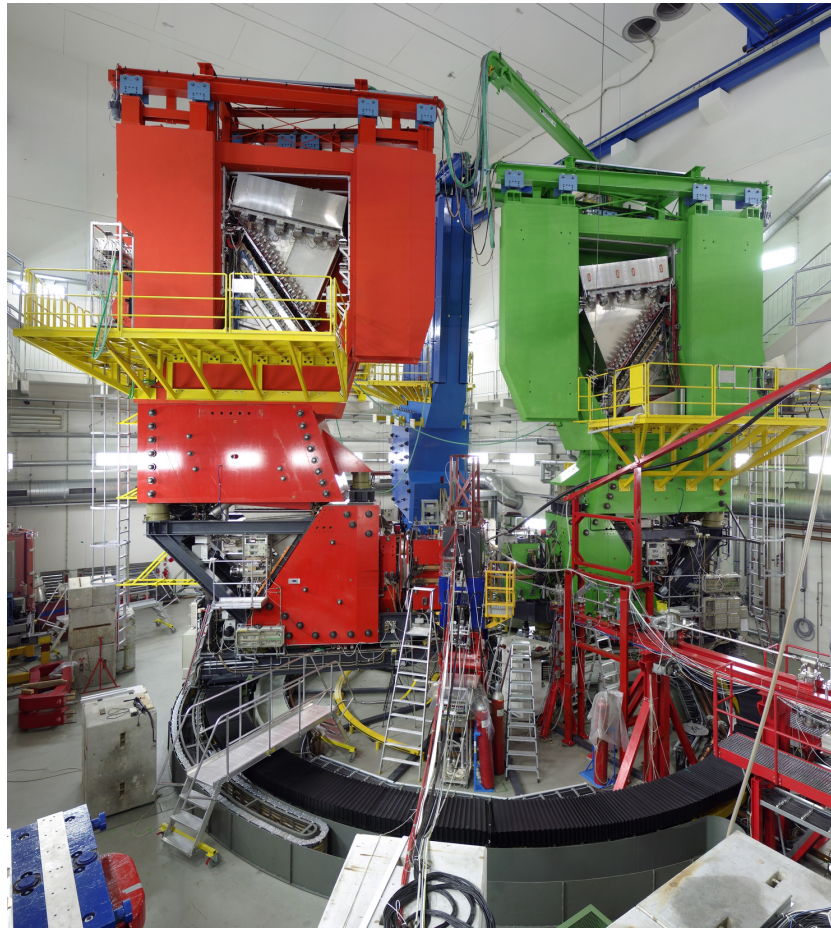
Figure 3.3 — The experimental hall of A1 collaboration. The name of the spectrometers, from left to the right, are A (red), B (blue) and C (green). In the middle of the photo is the SOS, placed in front of the target. The electron beam pipe is coming from the right side.
