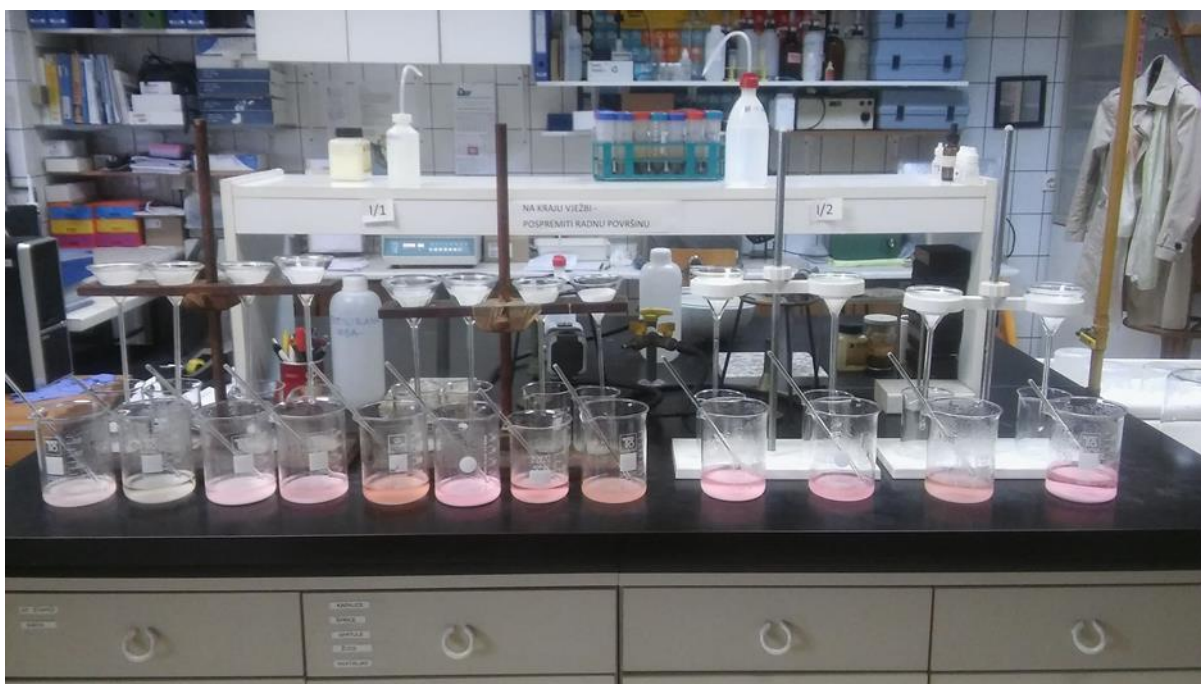
Figure 12. Filtration of solution containing \text{BaSO}_4 .
