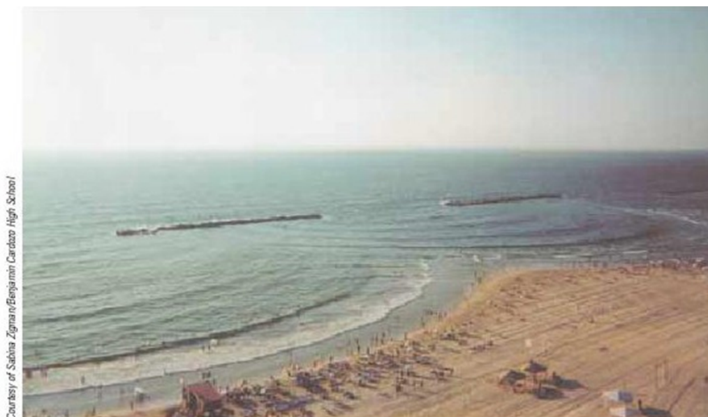
At a beach in Tel Aviv, Israel, plane water waves pass through two openings in a breakwall. Notice the diffraction effect—the waves exit the openings with circular wave fronts, as in Figure 37.1b. Notice also how the beach has been shaped by the circular wave fronts.
