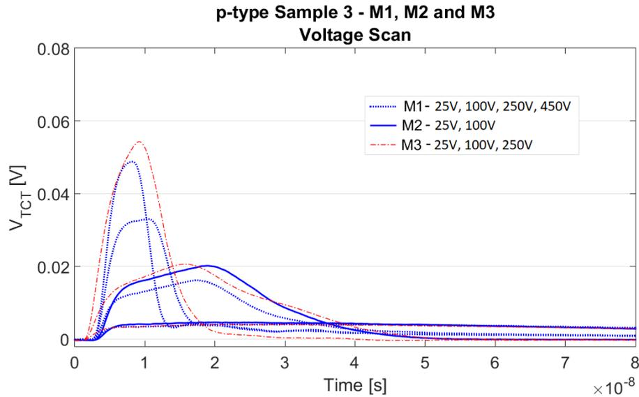
Figure 6.2: TCT voltage scan with red laser at 25, 100, 250 and 450 V. Plot presents signals from the p-type Sample 3 obtained in M1, M2 and M3 measurement conditions.
