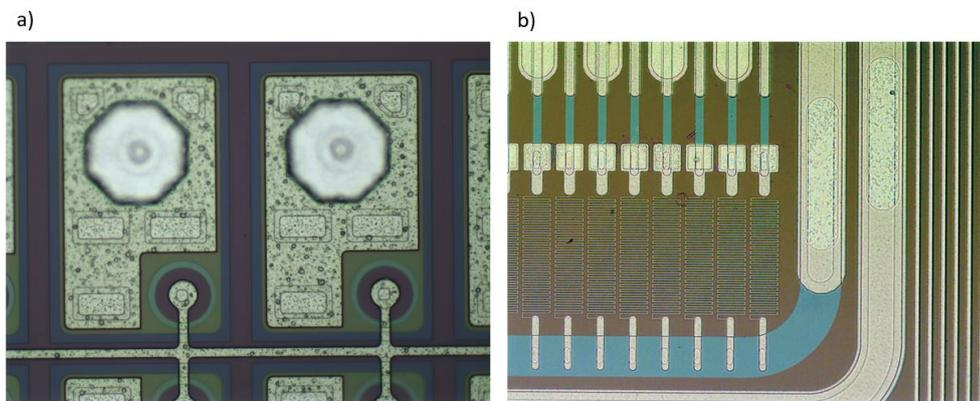
Figure 2.11: Photographs show: a) CMS pixels; b) strip detector. The CMS pixel dimension is  $120\mu\text{m} \times 150\mu\text{m}$  and strip width is  $20\mu\text{m}$ . [photographs courtesy of J. Härkönen]
