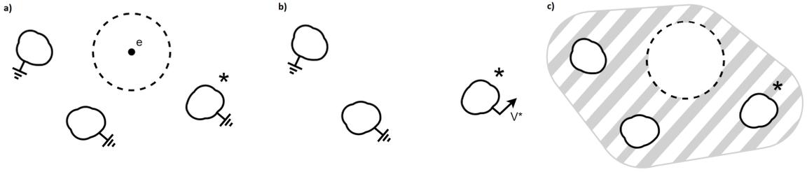
Figure D.1: a) Case A. Charge carrier is moving in otherwise empty space between grounded conductors. b) Case B. There are no charge carriers. One conductor (\*) is raised to unit potential, others are grounded. c) Volume under consideration in the Green's theorem.
