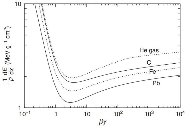
Figure 2.6: The ionisation energy loss curves for charged particles with  $Z = 1$  traversing lead, iron, carbon and gaseous helium. The  $\beta\gamma$  is equal to  $p/mc$ , where  $p$  is particle momentum and  $m$  is particle rest mass. Energy is related to momentum according to relativistic equation  $E^2 = (pc)^2 + (mc^2)^2$  [12].
