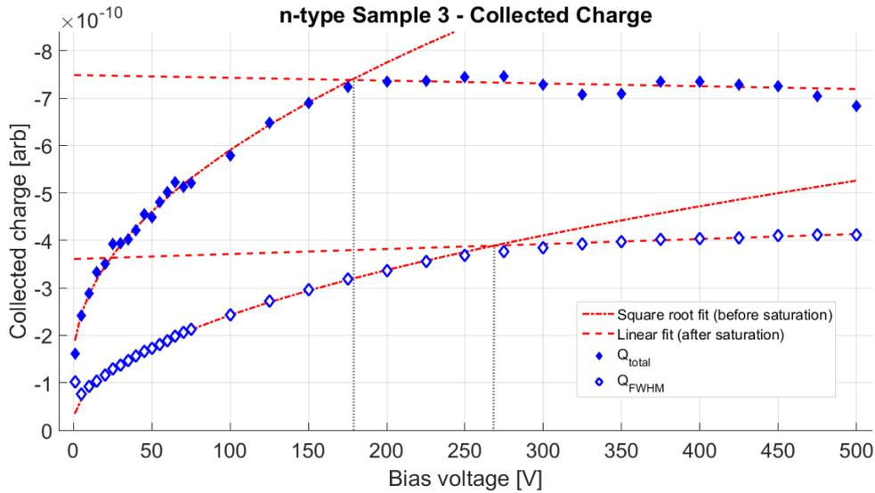
Figure 6.3: The plot shows the collected charge contained in the total pulse ( $Q_{total}$ ) and within FWHM of the pulse peak ( $Q_{FWHM}$ ). A square root function was fitted on the data before saturation, and linear fit was applied to the data after saturation. Since the FWHM integration causes some charge loss, saturation was slower and the point of full depletion was artificially higher. The plot presents data from Sample 3 M1 measurement.
