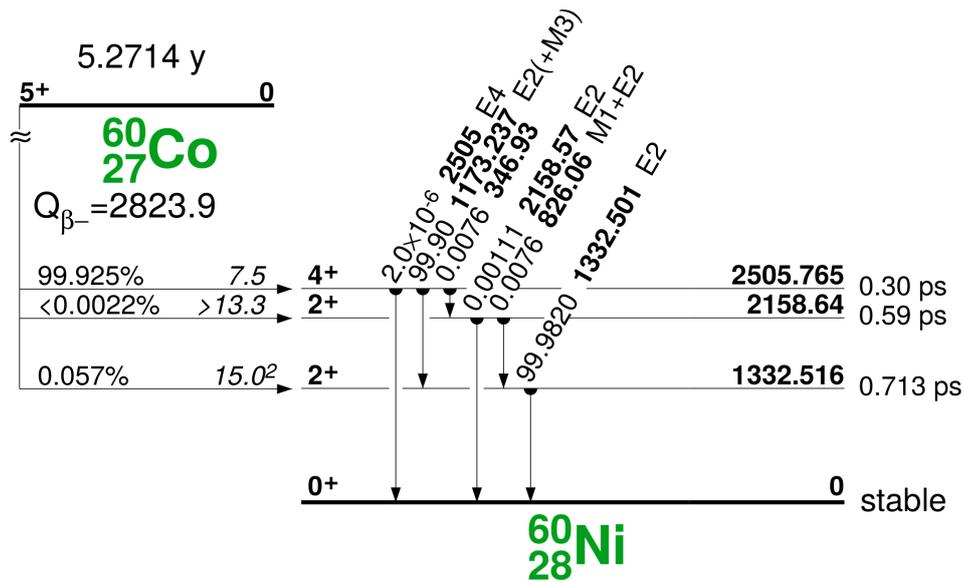
Figure 5.1: Basic decay scheme of  $^{60}\text{Co}$  [41].
