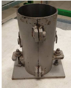
Figure 3.5 Cylindric mould (100 × 200) mm dimensions
