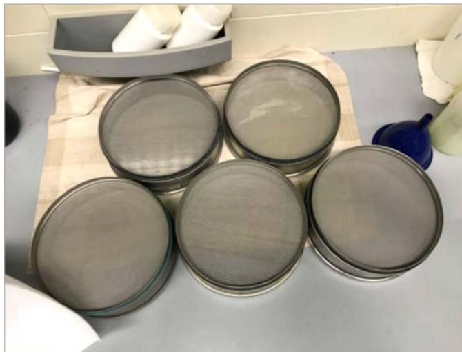
Slika 6. Standardna Retsch®ASTM sita
