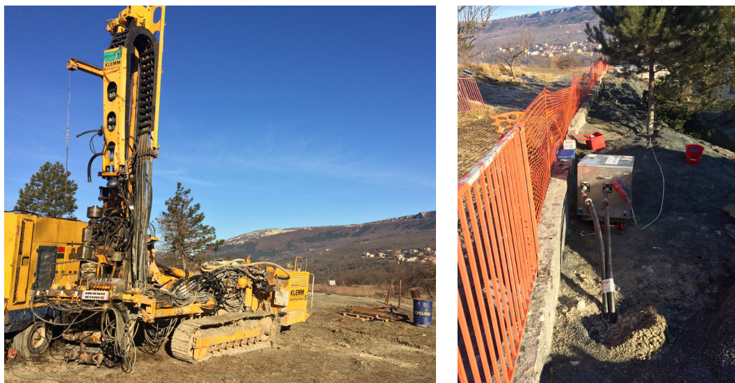
Figure 3: left) Experimental test site – drilling operations; right) Thermal response test equipment during testing
