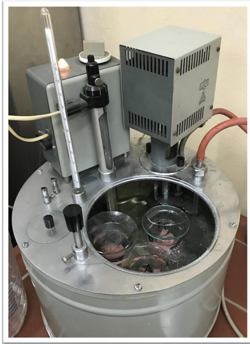
Figure 6. Water bath at 37 °C used for storing specimens before testing
