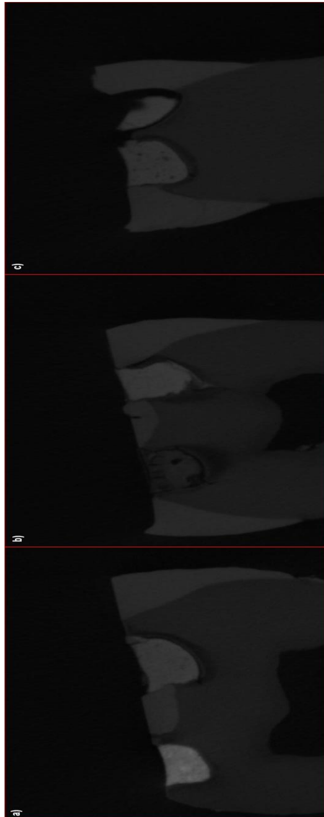
Figure 34. Micro-CT scan taken following the 45-day incubation period a) EQUIA Forte® HT and GC Fuji TRIAGE, b) Riva Self Cure and Biodentine™ c) Cention Forte and composite material.
