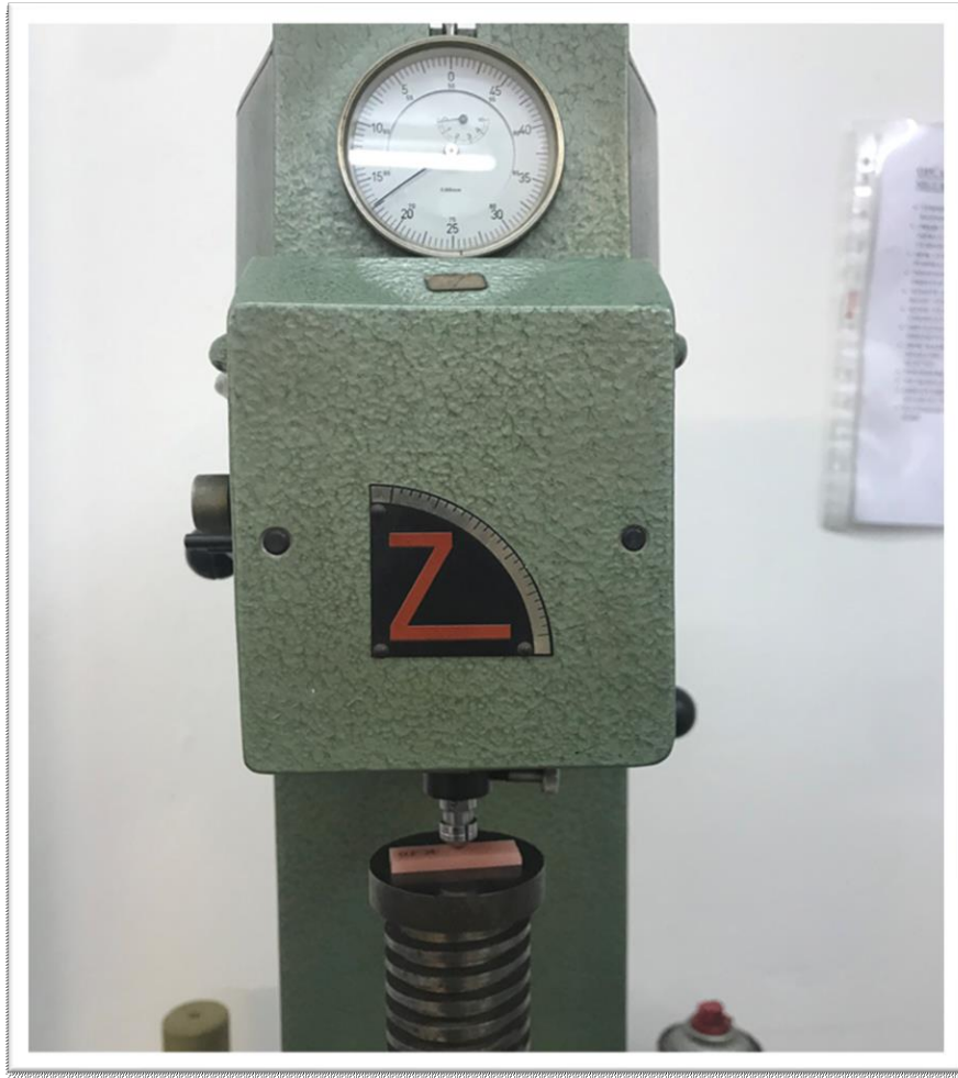
Figure 4. Zwick apparatus used for surface hardness testing
