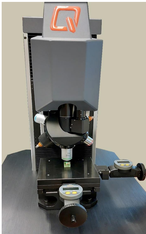
Figure 19. Dentine microhardness analysis.
