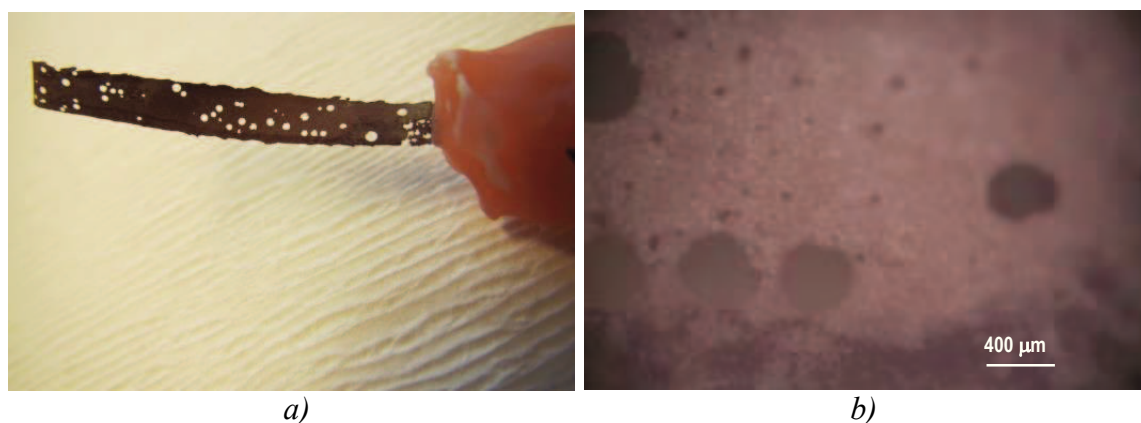
Figure 7. Cu-Al-Ni electrode after polarization measurements in 0.9% NaCl solution, T = 24 \text{ oC} , \text{pH} = 7.4 : a) macro image and b) light microscope image with magnification of 50 times.
